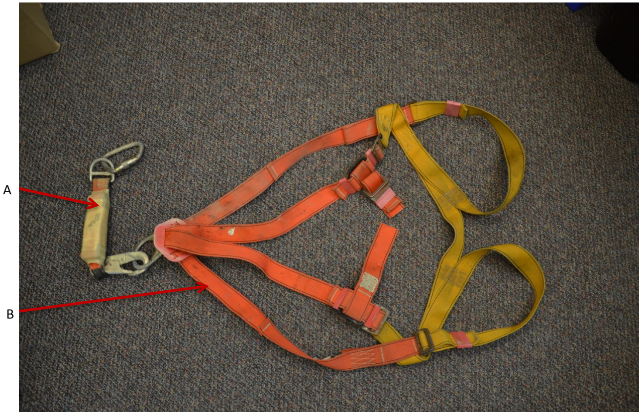
Figure 4. The full body harness and the shock absorbing lanyard from the incident
