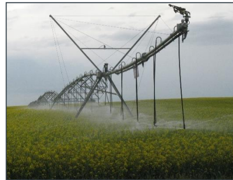
Canola crop being irrigated by a center pivot irrigation system.
