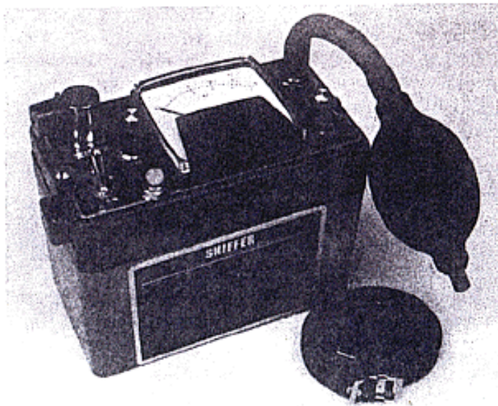
Figure 5-13 This is an example of an Oxygen meter with an aspirator bulb.
