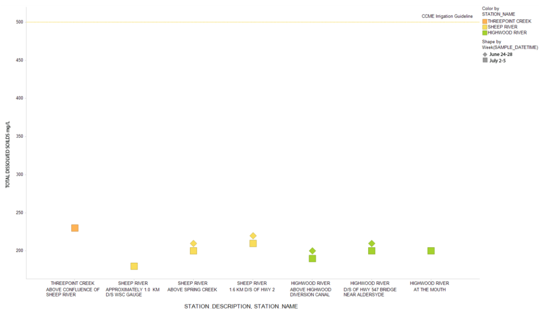
Figure 17. Total Dissolved Solids measured at Highwood River, Sheep River and Threepoint Creek sites.
