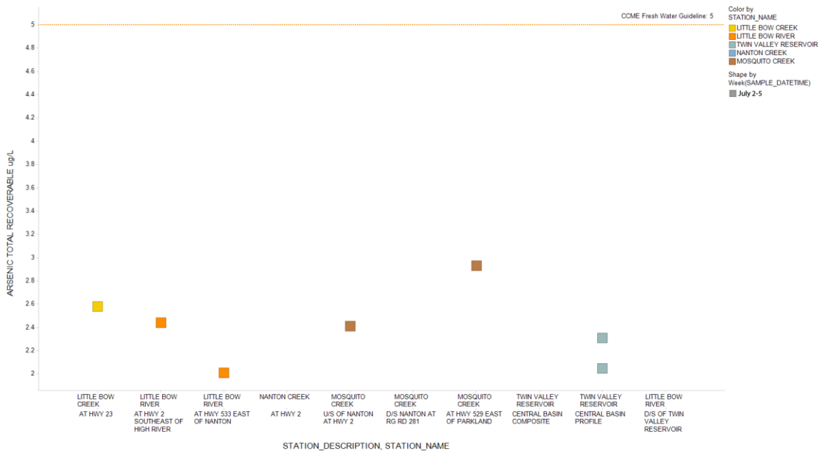
Figure 34. Total Arsenic measured at Little Bow River, Mosquito Creek and Twin Valley Reservoir sites.
