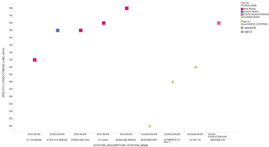
Figure 7. Electrical conductivity (specific conductance) measured at Bow, Oldman and South Saskatchewan river sites.
