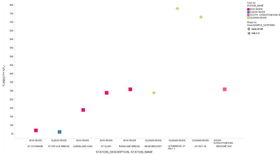
Figure 8. Turbidity measurements at the Bow, Oldman and South Saskatchewan river sites.
