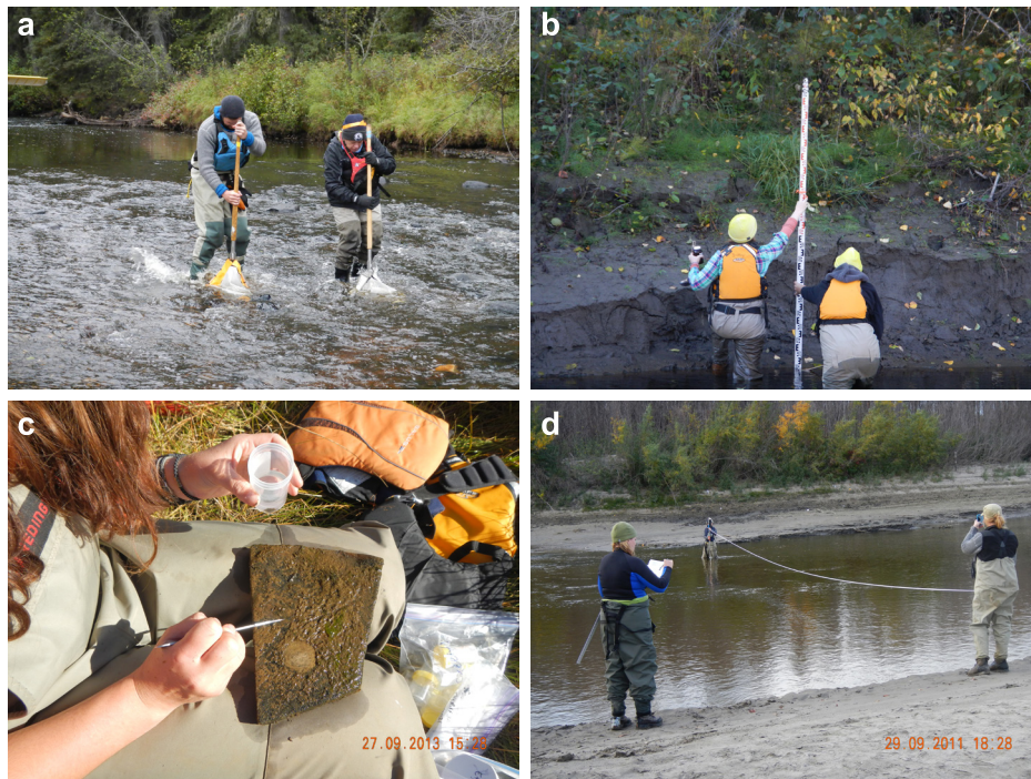
Figure 13. Examples of sampling methodology used in the tributaries of the Lower Athabasca River benthic biomonitoring study: a) collection of kick net sampling for benthic invertebrates – here different mesh sizes are used to aid comparison of historical and contemporary samples; b) estimation of bank height as part of the Canadian Aquatic Biomonitoring Network (CABIN) procedures; 3c) collection of algal periphyton on hard substrate using the “scalpel-scraping” technique; and 3d) measurement of wetted width of sampling reach.
