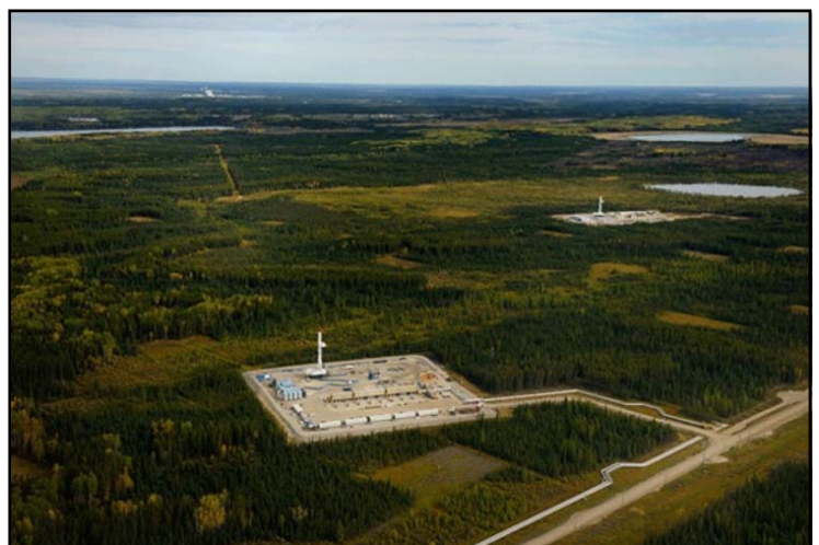
Well pads with SAGD drilling rigs at Cenovus Energy's Christina Lake oil sands operation in northern Alberta.
