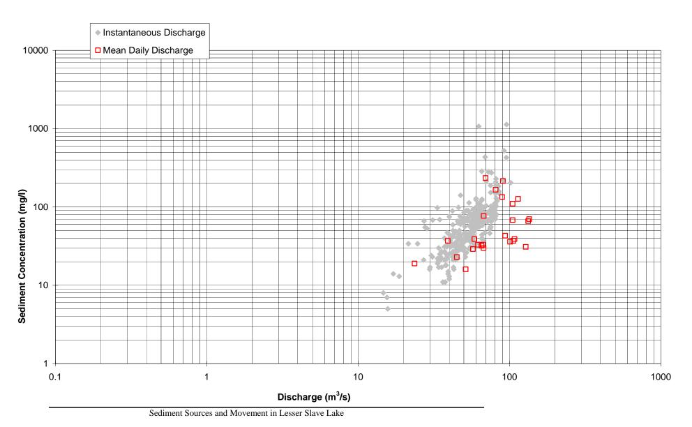
Fig 6: Sediment Rating Curve for the Lesser Slave River at Slave Lake, 1978 - 1997.
