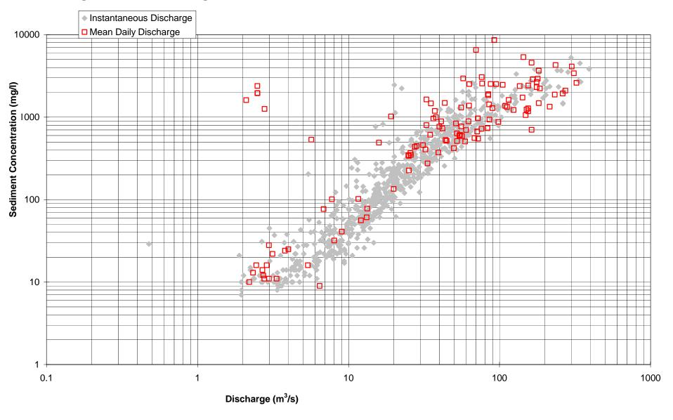
Fig 2: Sediment Rating Curve for the Driftpile River at Driftpile, 1977 - 1986.
