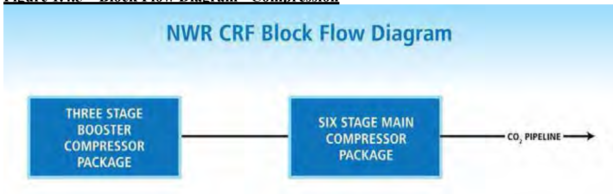
Figure 1.4.5 – Block Flow Diagram - Compression
