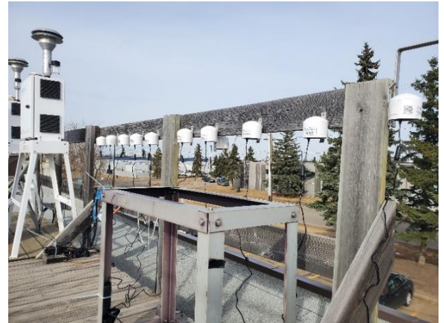
Figure 1: Ten PurpleAir sensors undergoing testing in Edmonton in March 2021, in preparation for the wildfire season.
