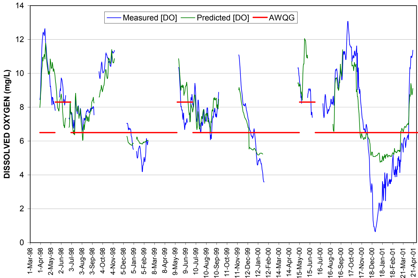
Figure 4.3 Predicted and observed dissolved oxygen concentrations at the Muskeg River WSC site, 1998-2001
