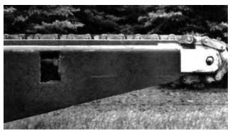
FIGURE 3. Conveyor Chain Adjustment.
