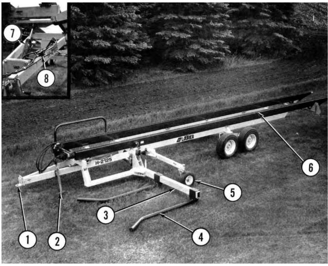
FIGURE 1. Laurier H-2125 Round Bale Mover: (1) Adjustable Hitch, (2) Hitch Jack, (3) Lift Arm, (4) Bale Forks, (5) Outrigger Wheel, (6) Conveyor Chains, (7) Deck Tilt Cylinder, (8) Hydraulic Valves.
