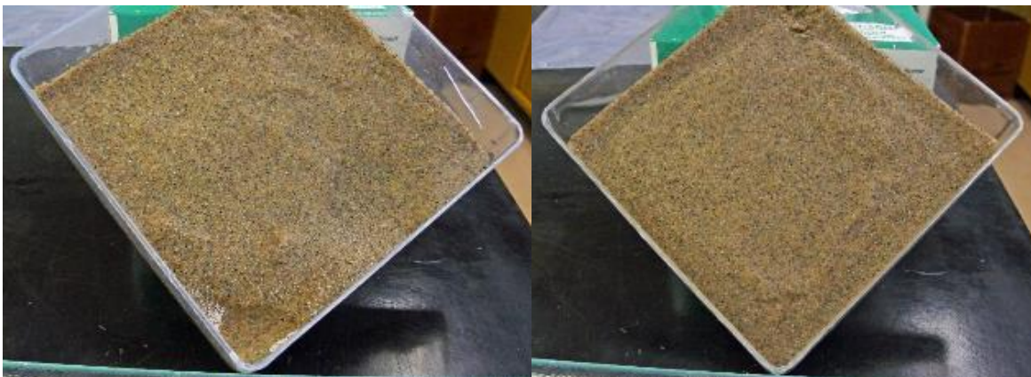
Figure 3: ISTA-approved clean sand medium showing too much water on left and correct water amount on right. When the correct amount of water is added, particles of sand should have the capacity to hold sufficient water to provide continuous movement of water to the seeds, but also provide sufficient pore space for aeration.
