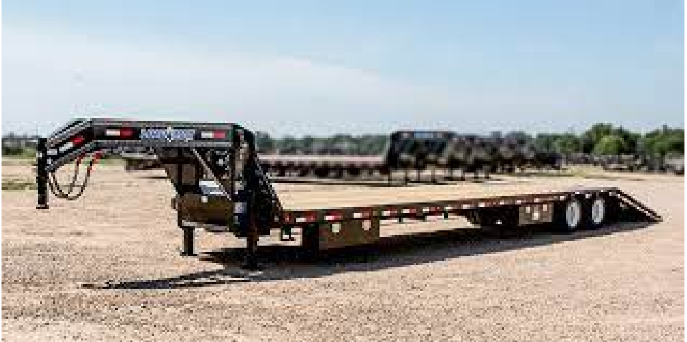
Figure 2. Represents what a gooseneck trailer would look like. Photo obtained from the web showing the type of trailer involved in the incident.
