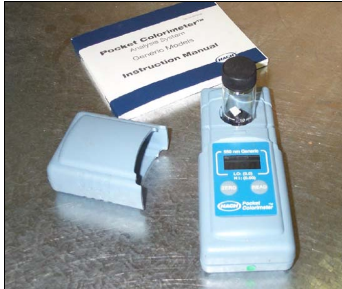
Figure 1. Hand-held colorimeter used for methodology of Weil et al. (2003)
