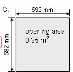
**Examples B and C conform** to height, width and area requirements.
