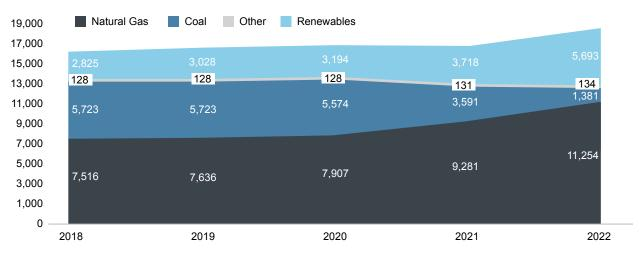
Natural gas generates the vast majority of Alberta's electricity at more than 11,000 megawatts (MW) of installed capacity, with cogeneration accounting for 5,438 MW of this capacity.
