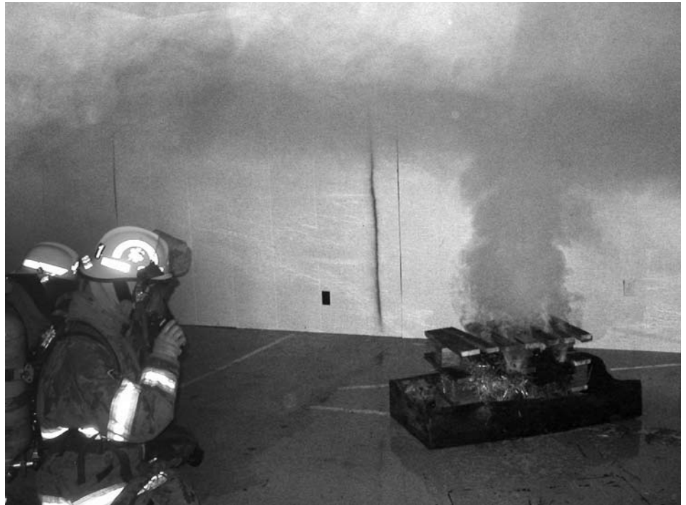
Firefighters conducting a smoke progression experiment
