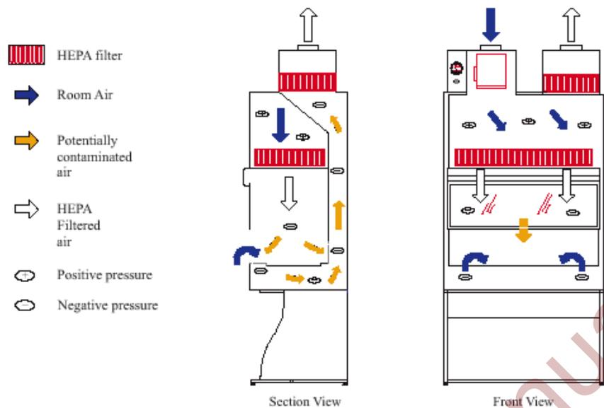
Proper use of BSCs is essential for the devices to function as they are designed.
