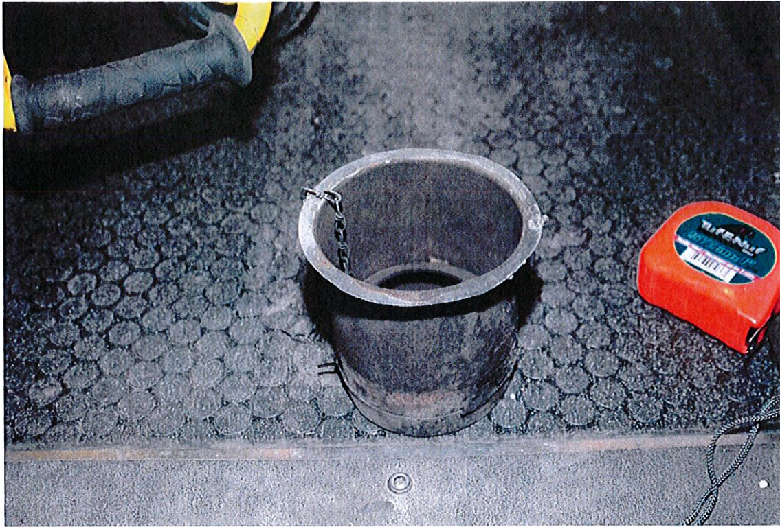
Photograph #7: Shows the fuel tank filler neck that struck the worker.
