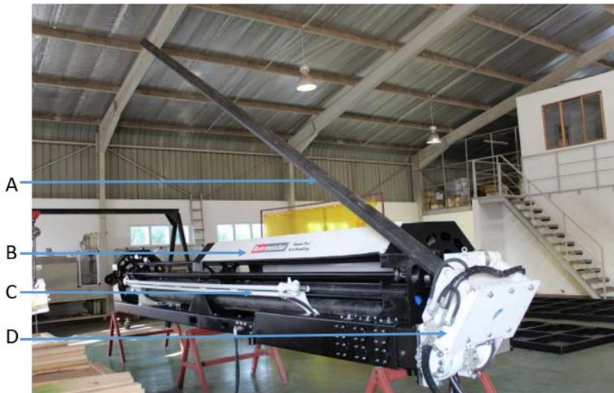
Figure 1. Bohrmeister rod handler. Image provided by Google Images.
