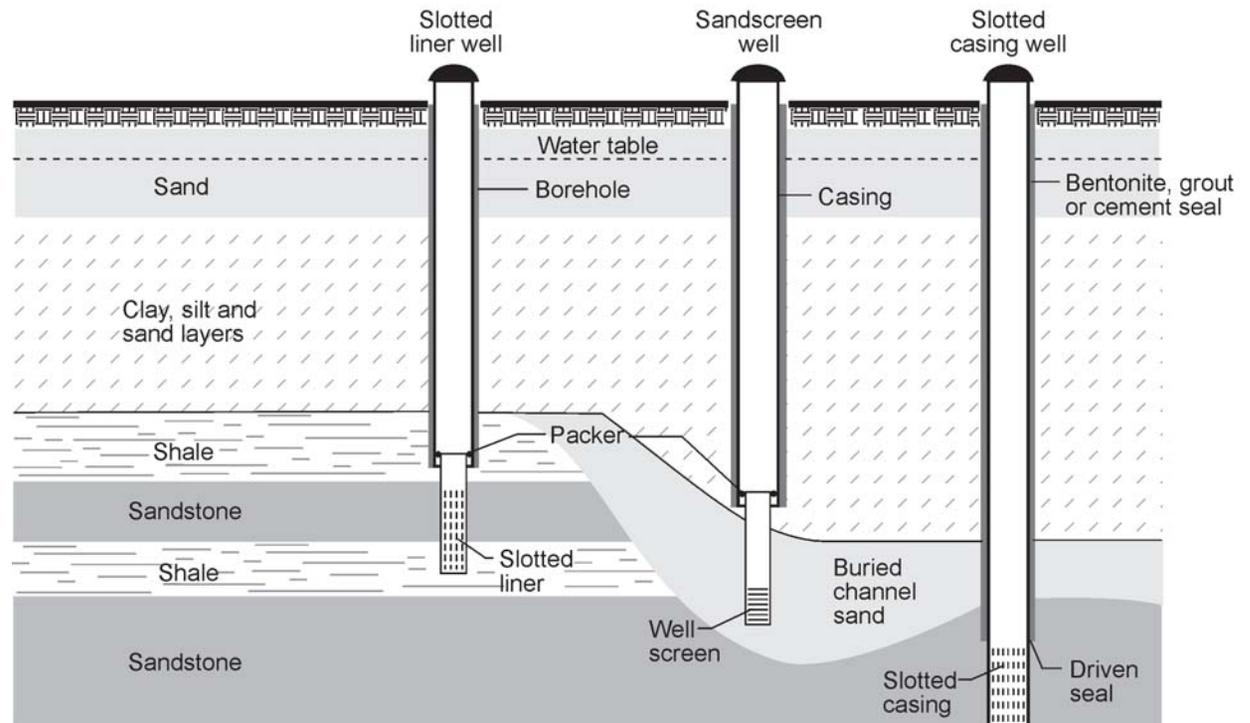
***Provincial regulations provide detailed specifications for casing diameters and wall thicknesses. All casing must meet or exceed standards set by the Canadian Standards Association or the American Society of Testing and Materials (see Appendix 1, "Water Well Casing Specifications" on page 33).***
