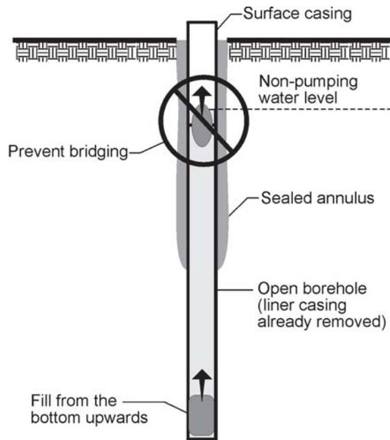
*By regulation, a well must be filled full length with impervious material. That material must be introduced into the well at the bottom and be placed progressively upward to ground surface.*
