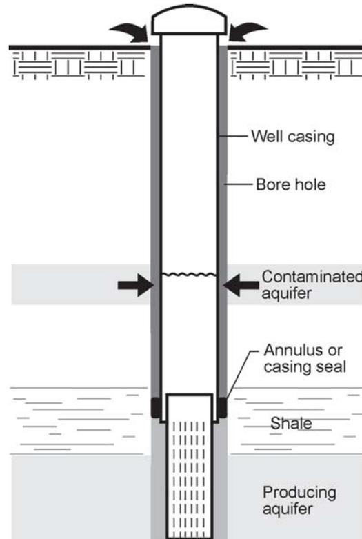
Figure 2 Multi-Aquifer Well Completion
