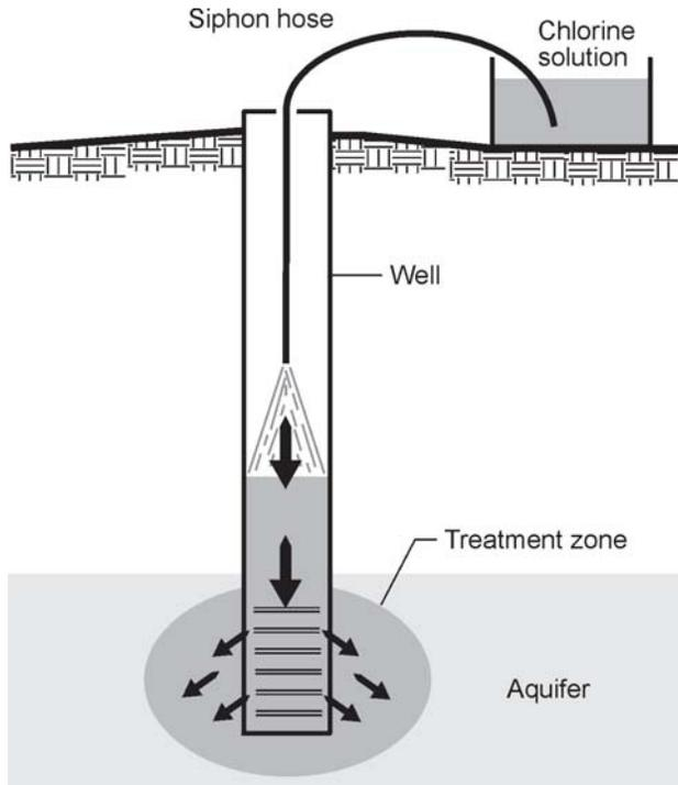
**Step 4** Siphon this solution into the well (see Figure 2, Siphoning Chlorine Solution).
