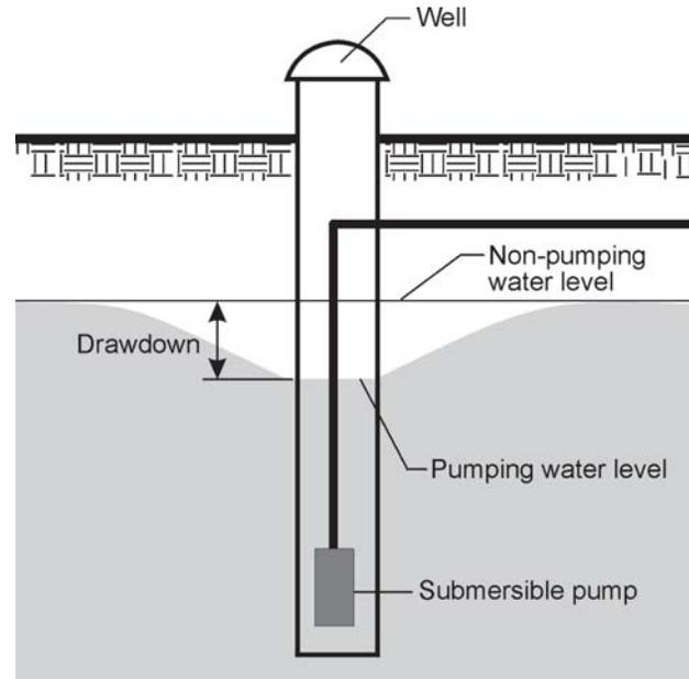
*Even when the pumping water level remains relatively steady, you need to do regular annual maintenance, including shock chlorination, to control bacteria buildup. If you allow a well to deteriorate for too long, it may not be possible to restore its original capacity.*
