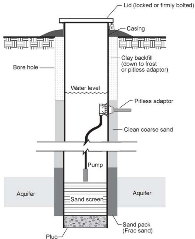
*Materials used in the drilling and construction of water wells must be new and uncontaminated.*
