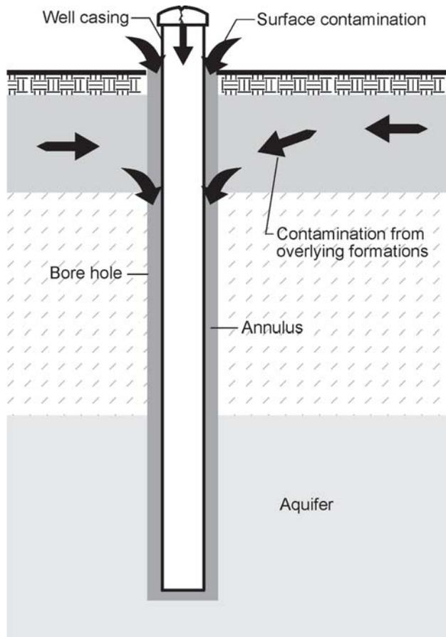
*Wells that are no longer being used should be plugged. They are a serious public safety and environmental hazard.*
