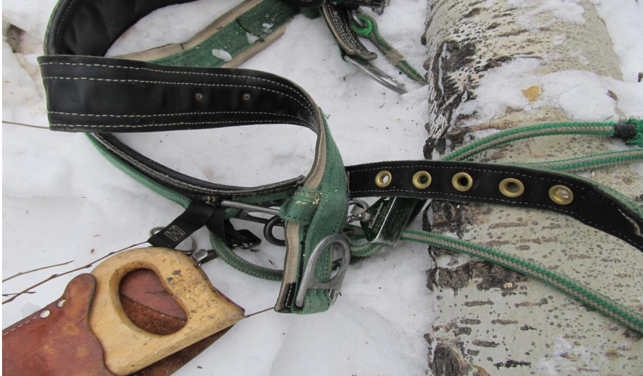
Figure 2. Unbuckled work positioning harness.
