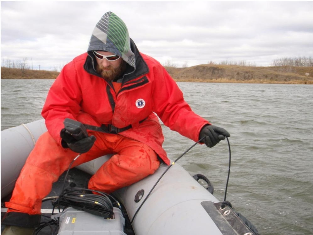
Figure 46. Black Nugget Mine Pit Lake (October) – sampling with YSI meter from Zodiac.
