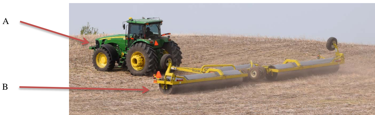
Figure 2. Similar tractor and land roller working at incident site. Photo shows land roller in deployed configuration
