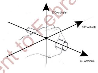
Figure A2 – Axes for Measurement of Hand-Arm Vibration (Adapted from the Hand-Arm Vibration Guide, Griffin et al, 2006)
