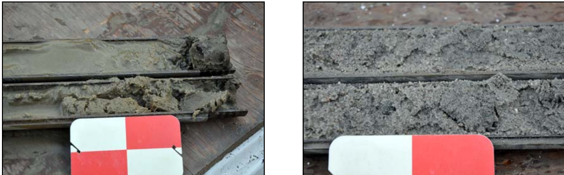
Figure 13: Image to the left shows the fine saturated brown sand collected from the first water bearing unit (6.4-6.7 m). To the right shows a medium to coarse grain saturated grey sand collected from the second water bearing unit (9.2-9.8 m). Rectangles in the scale card are 2 x 5 cm.
