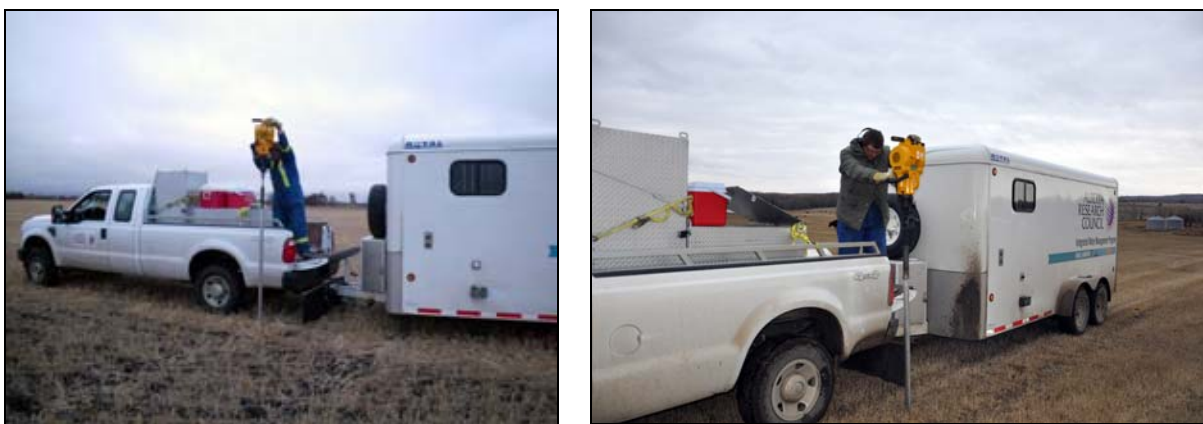
Figure 6: Core collection using a pionjar drill from the field applied drill cuttings (left) and the field applied fertilizer (right).
