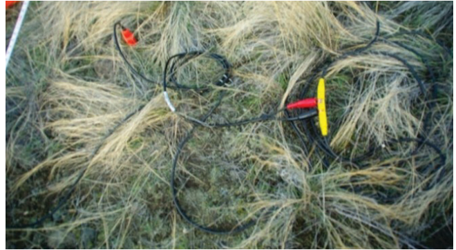
Photo: Typical seismic geophone placement.
