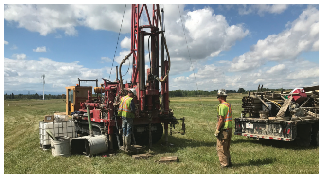
Example track-mounted rotary drill rig with water tank (left) and support truck (right).
