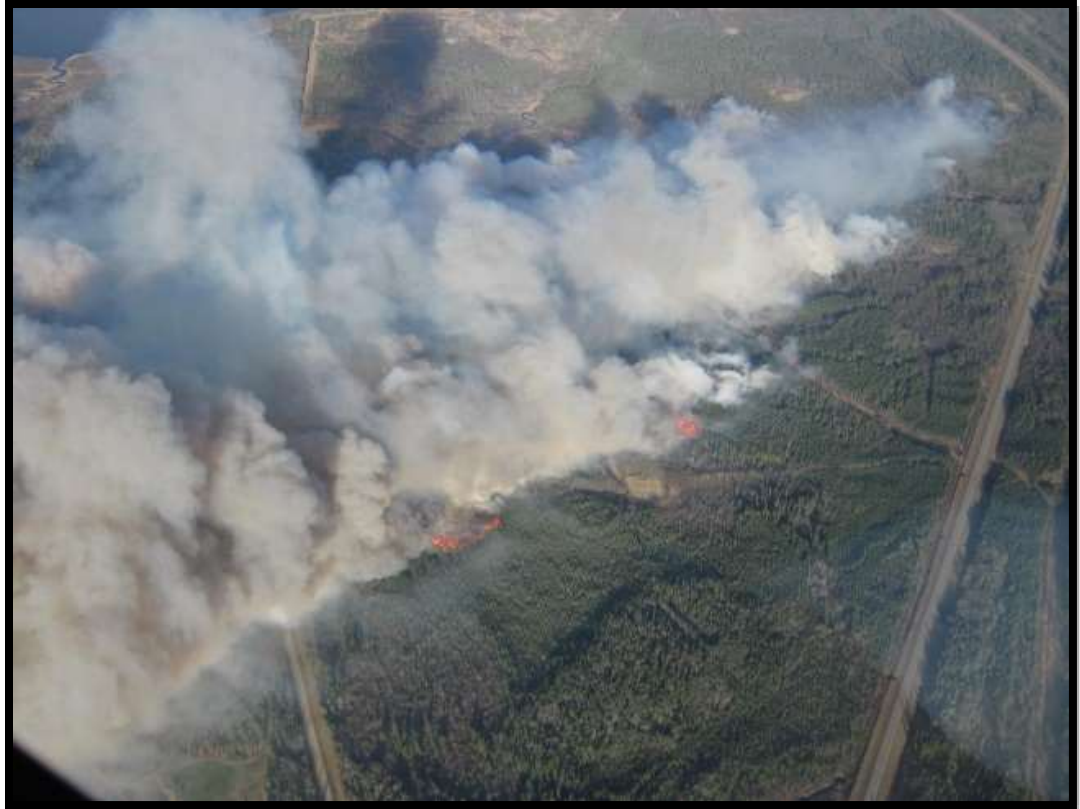
Figure 48 – Illustration of a typical wind-driven wildfire with short-range spotting and low smoke drift directly ahead of the fire front.
