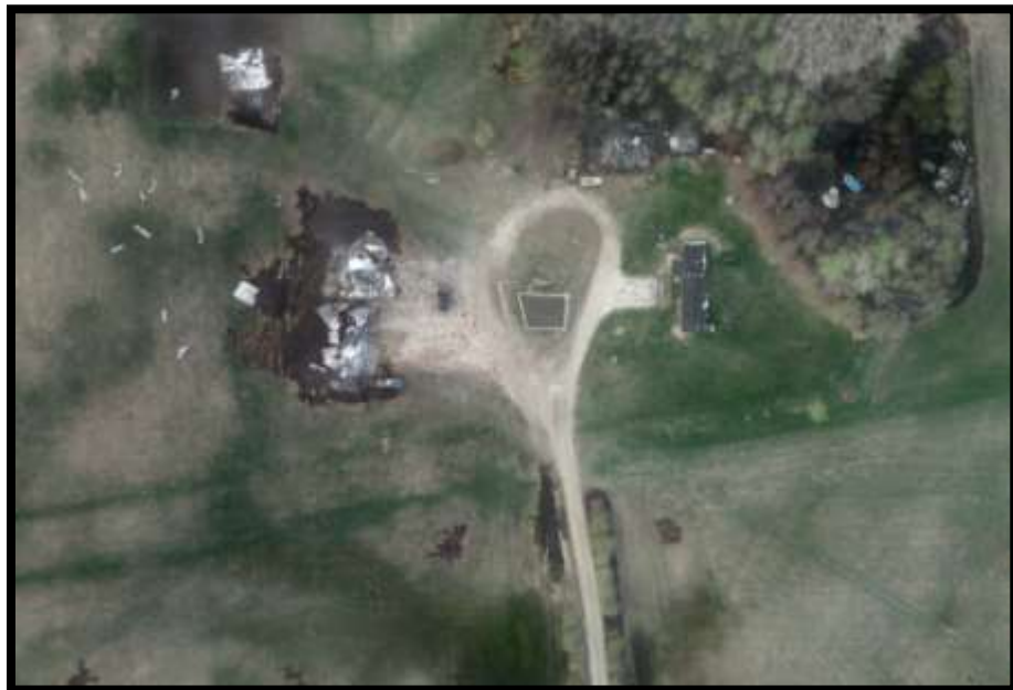
Figure 128 – Ember transport (spotting) ignited homes independent of surface fire spread.
