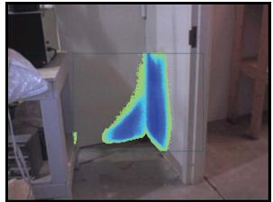
Infrared View of Wet Drywall
