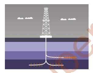
\* Re-fractures of existing well legs and additional well lengthening is represented by orange
