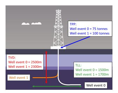
\* A new leg (i.e., well event 1) is represented by orange, and example figures for TVD, TLL and TPP are included for the example calculation above.
