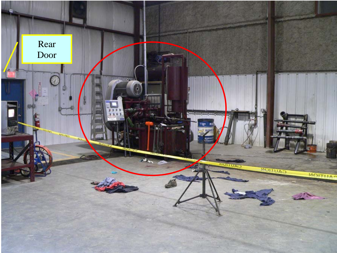
Photograph #1 Shows the progressive cavity pump test bench located in the northeast corner of the pump shop (circled in red).
