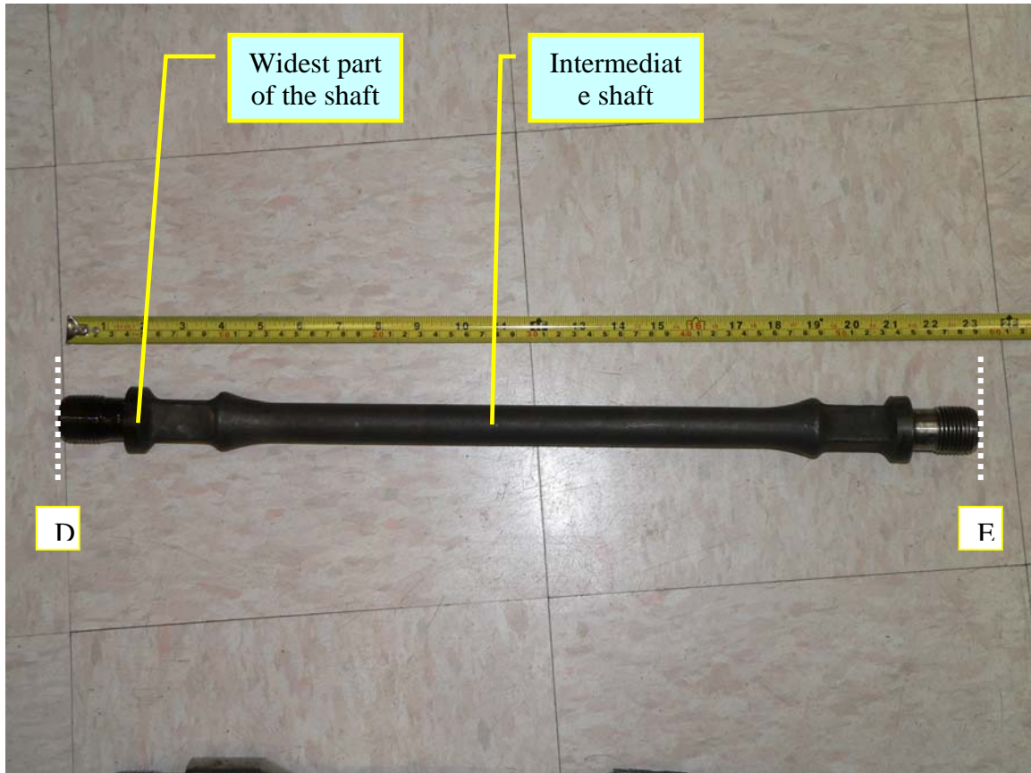
Photograph #8 Shows the second pony rod that attached to the rotor of the progressive cavity pump. It measured 580 mm in length from D to E. This measurement includes the thread length hidden inside the adapter. The threaded end at the widest part measured 40 mm. The ends were also designed to fit a 23 mm wrench. The intermediate or middle shaft measured 25 mm in diameter and was made of steel material.
