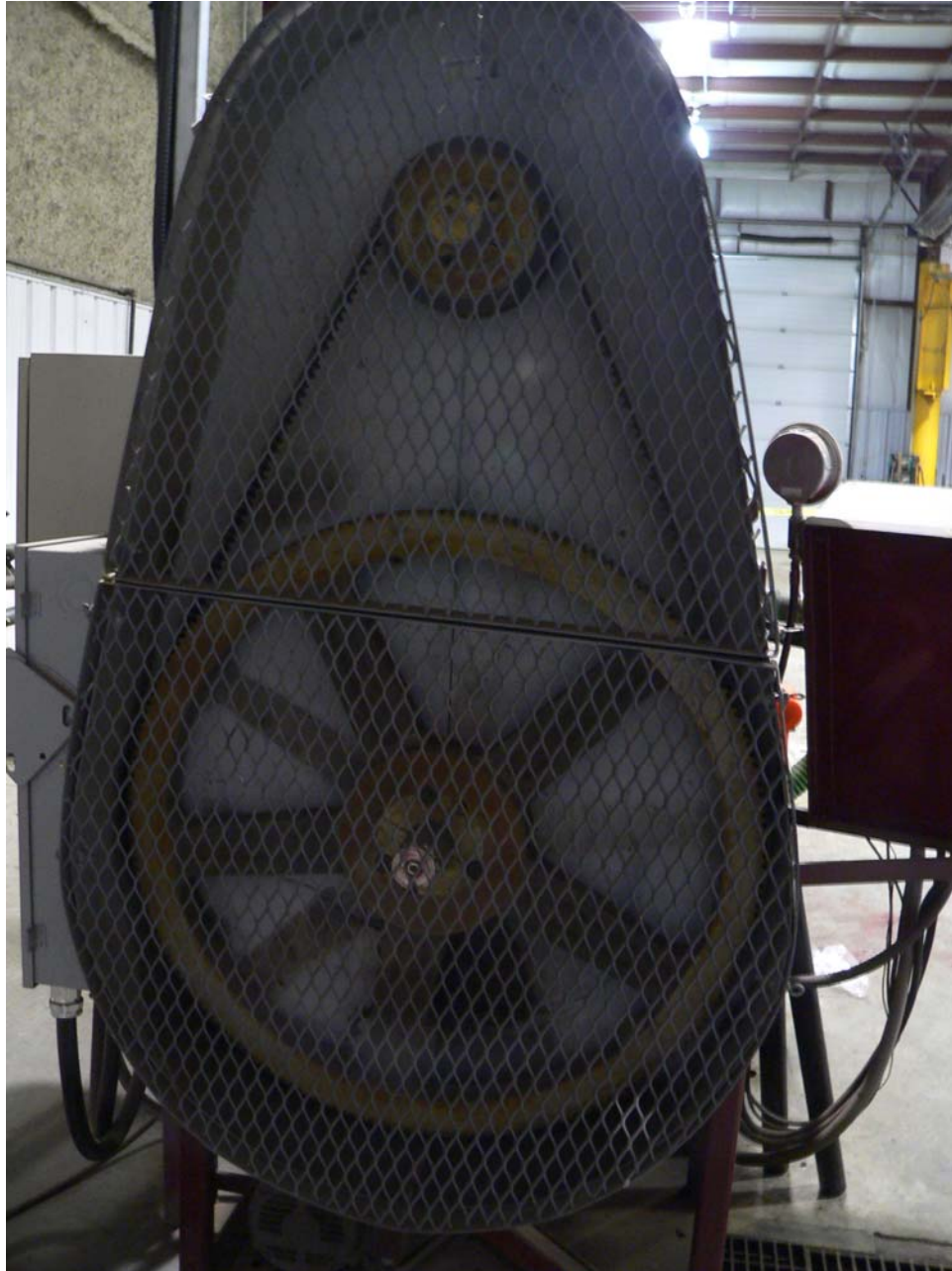
Photograph #5 Shows the right side of the progressive cavity test bench. The flywheel enables the polish rod to rotate at the maximum 300 revolutions per minute (rpm) and 1330 ft-lbs of torque.
