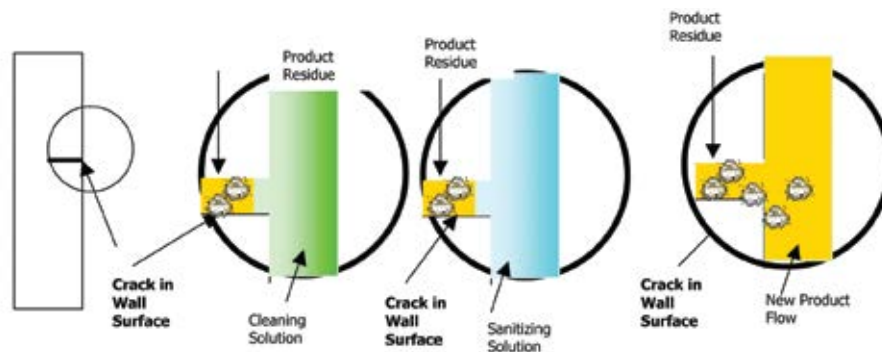
Figure 1: How Joints, Cracks, or Crevices in Tanks and Pipes Reduce or Limit Operation of CIP Systems
