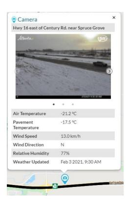
The Road Weather Information Stations (RWIS) provide both camera images and weather information. This information helps to determine what maintenance activities may be needed for both current and forecast weather.
