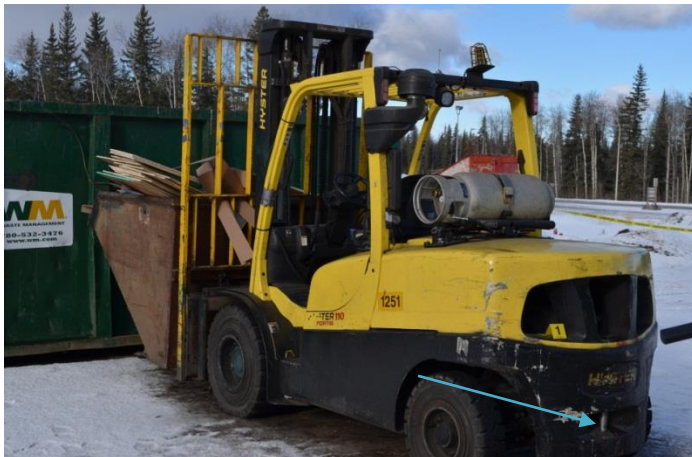
Figure 2. The blue arrow shows the area in which the Loader Operator was hooking the cable to the forklift at the time of the incident.
