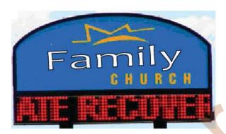
An electronic changeable copy sign is defined as a sign or portion thereof that displays electronic, non-pictorial, text information in which each alphanumeric character, graphic or symbol is defined by a small number of matrix elements using different combinations of light-emitting diodes (LEDs), fibre optics, lightbulbs or other illumination devices within the display area.
