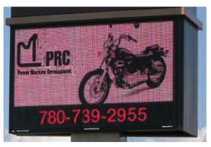
An electronic graphic display sign is defined as a sign or portion thereof that displays electronic, static images, static graphics or static pictures, with or without information, defined by a small number of matrix elements using different combinations of light-emitting diodes (LEDs), fibre optics, light bulbs or other illumination devices within the display area where the message accomplished change sequence is immediately or by means of fade. repixalization or dissolve modes.
