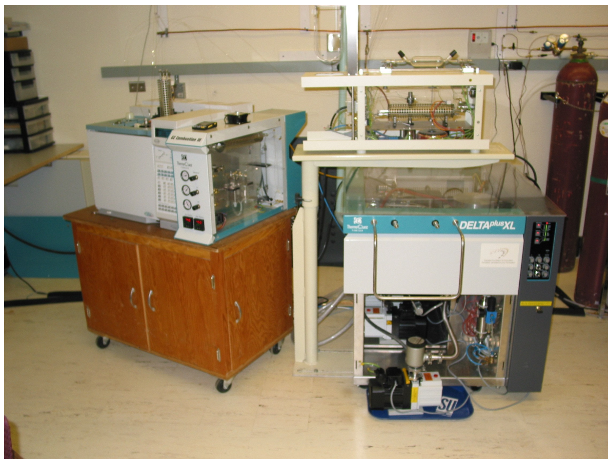
Figure 18: Analytical setup for carbon isotope ratio determinations in the Isotope Science Laboratory at the University of Calgary showing a gas chromatograph (left) and a cryo-focusing system (top right) interfaced with an isotope ratio mass spectrometer (bottom right).
