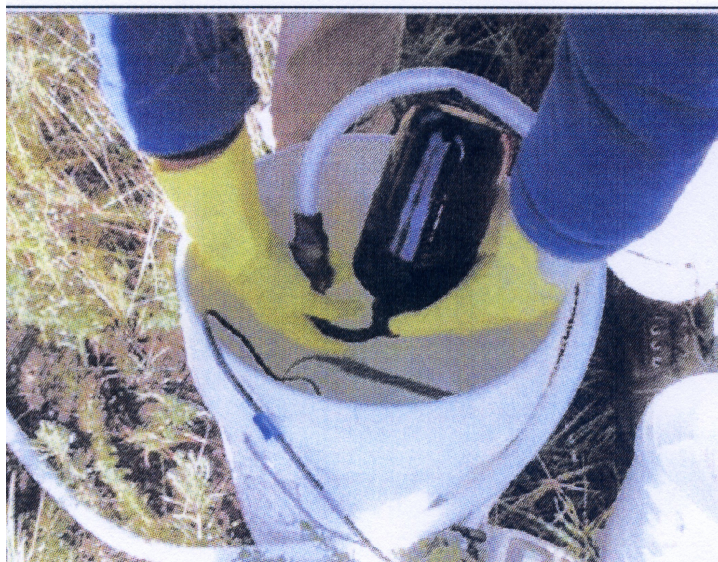
Figure 12: Sampling groundwater and its dissolved gases in an inverted 1-L Boston round bottle for subsequent extraction and chemical and isotopic analyses (photograph provided by Dr. A. W. Gorody, Universal Geoscience Consulting, Inc., Houston, Texas: from Gorody, 2006).
