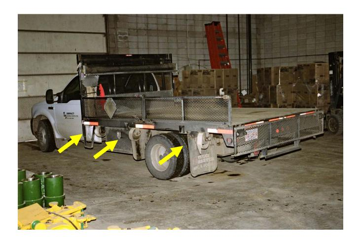
Photograph #1 Shows the flatbed truck in the Cando Oilfield Supply & Rentals Ltd. loading bay at 2104-8 Street, Nisku, Alberta. Arrows indicate the load securing strap reels fitted to the driver's side of the truck.
