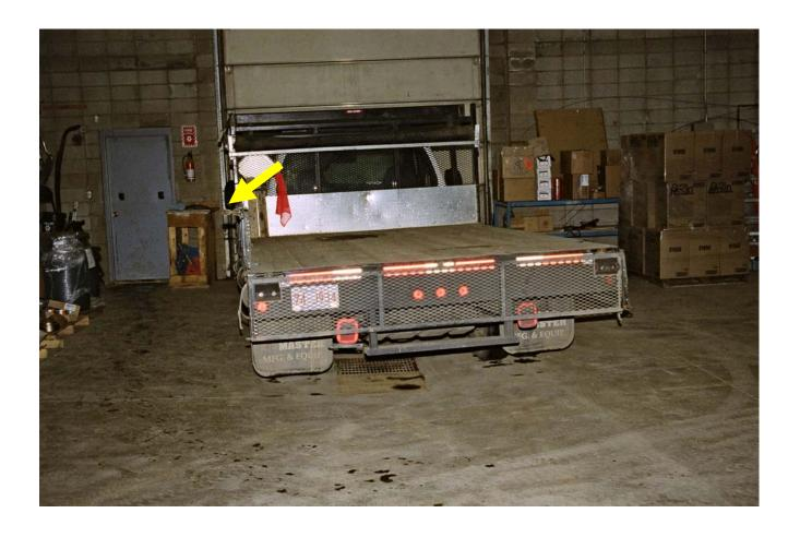
Photograph #2 Shows the flatbed fitted to the truck. Arrow shows pieces of 2x4 used to prevent load straps from deforming the load.
