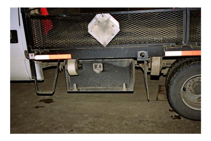
Photograph #4 Shows a close-up view of the two front load securing strap reels on the driver's side of the truck.
