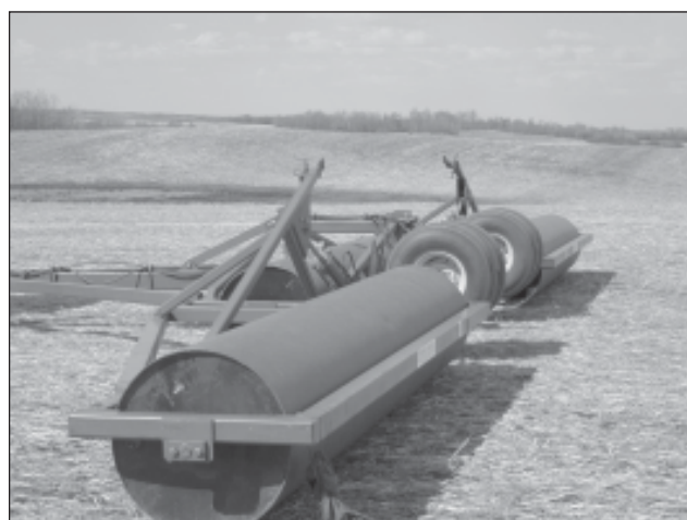
Figure 1. Roller used for land rolling pulse crops.
