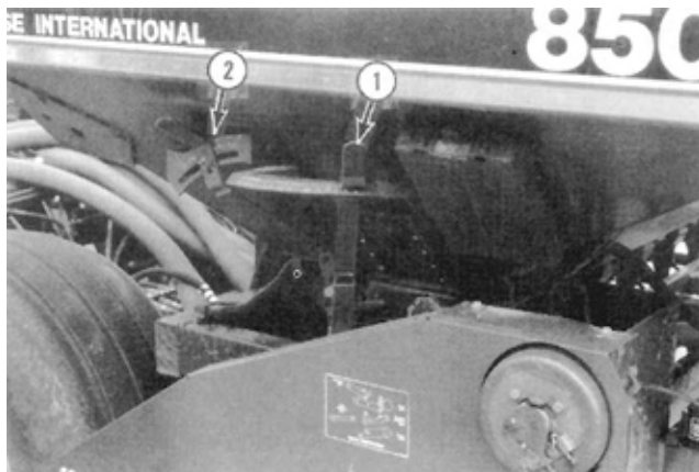
FIGURE 19. Application Rate Adjustment: (1) Seed and (2) Fertilizer.
