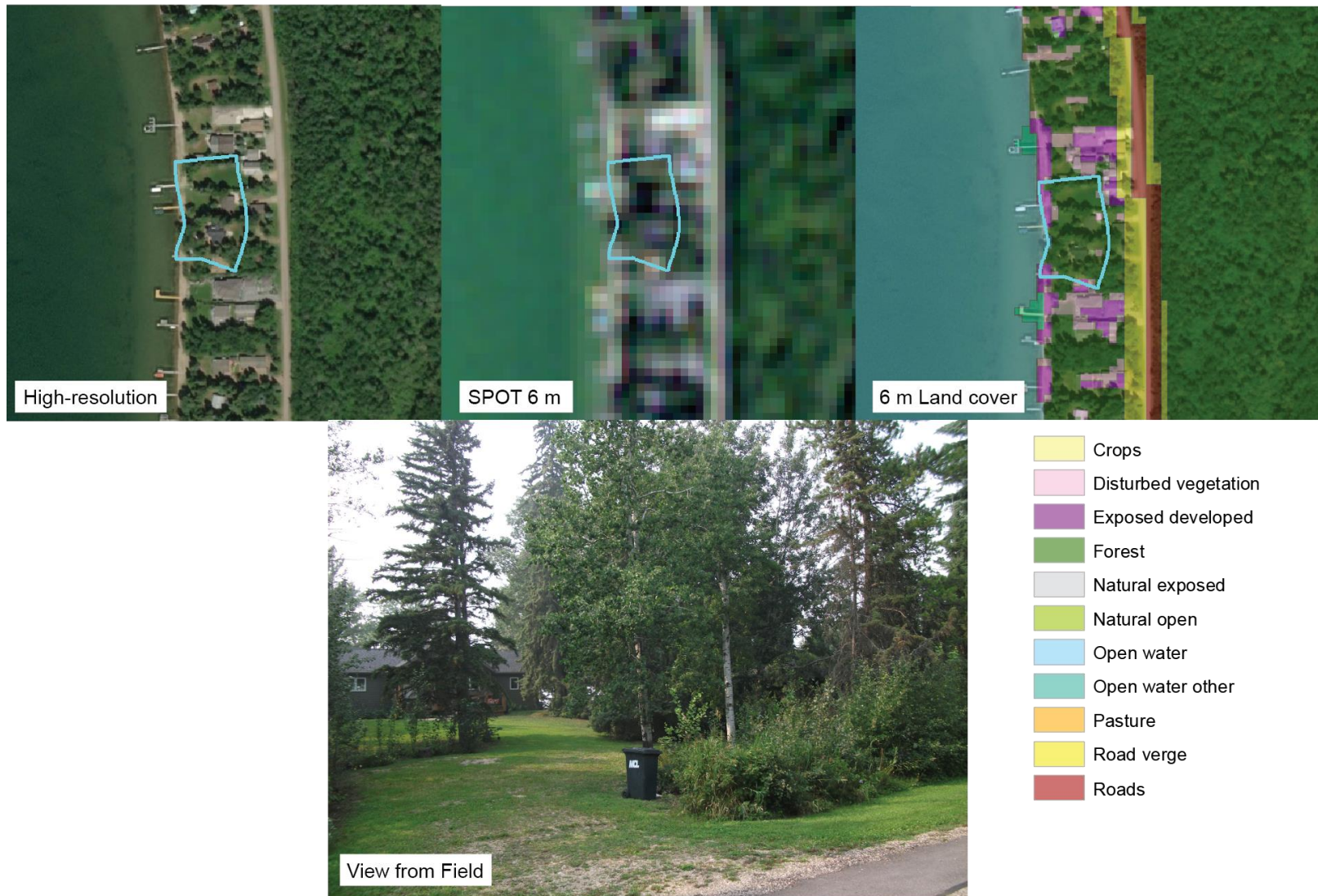
Figure 5. RMA U79 at Pigeon Lake. This RMA was assigned to the High category by the GIS tool, but was assigned to the Moderate category during the field assessment. In this instance, the error could be attributed to the SPOT image resolution, which resulted in the misclassification of human footprint as Forest.
