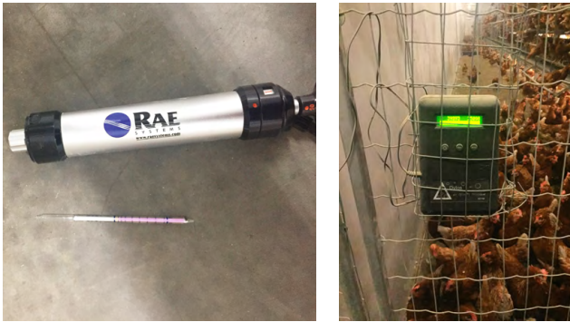
Figure 1. RAE gas detection pump and dosi-tube (left); Dylos DC1700 dust monitor (right)
