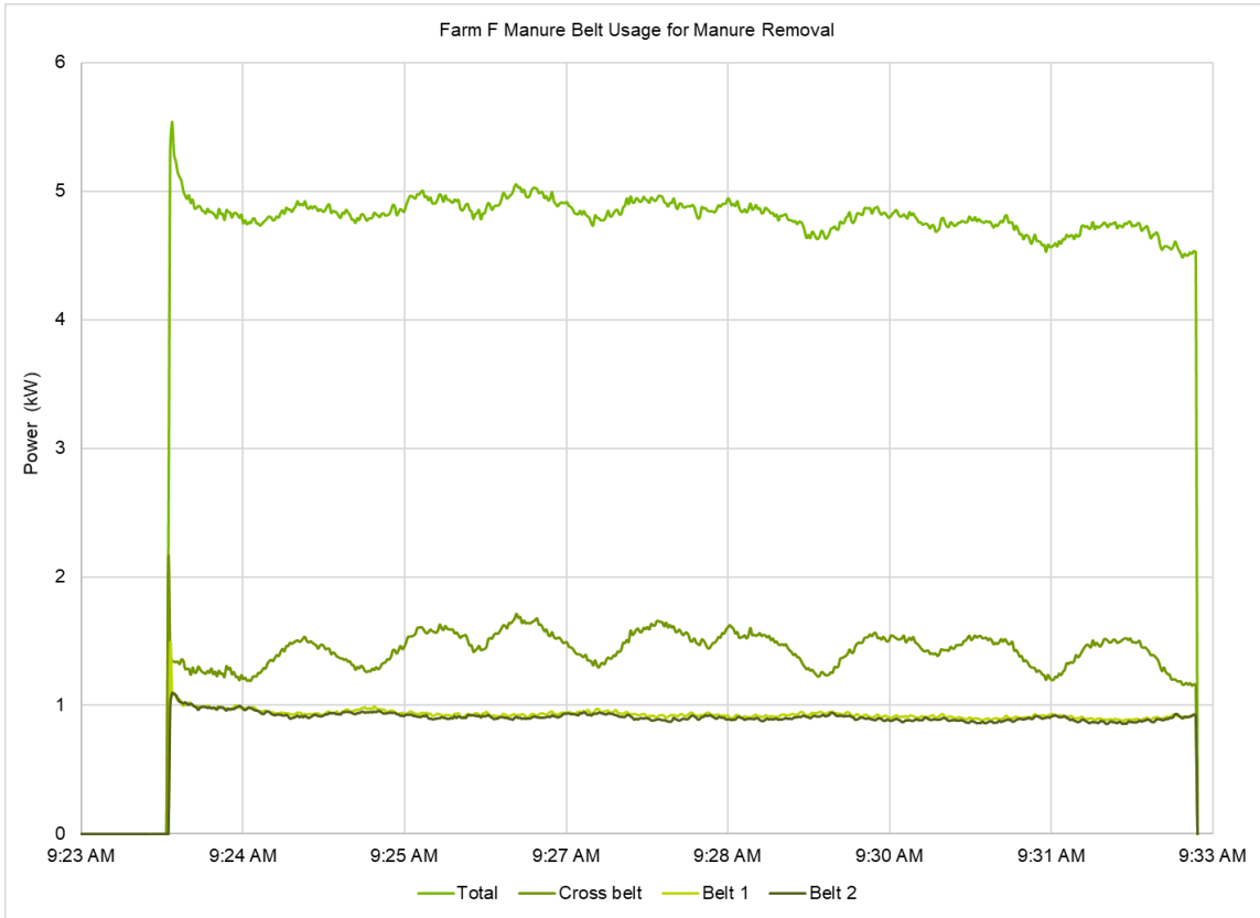
Figure 14. Example of energy consumption of manure belts while emptying at Farm F. The total energy was calculated for all four rows of belts as only two of the rows were monitored.
