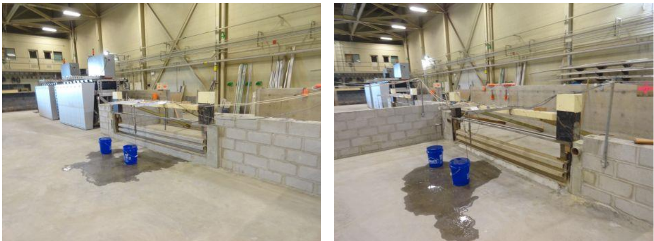
Figure 36. Diversion channel control weir (left) and main channel control weir (right).
