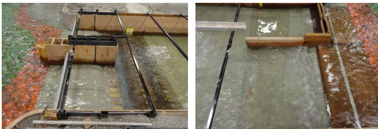
Figure 151. Flow conditions at the structure during the 320 m 3 /s event. Top – facing southwest at the diversion, bottom - facing southeast at the service spillway.
