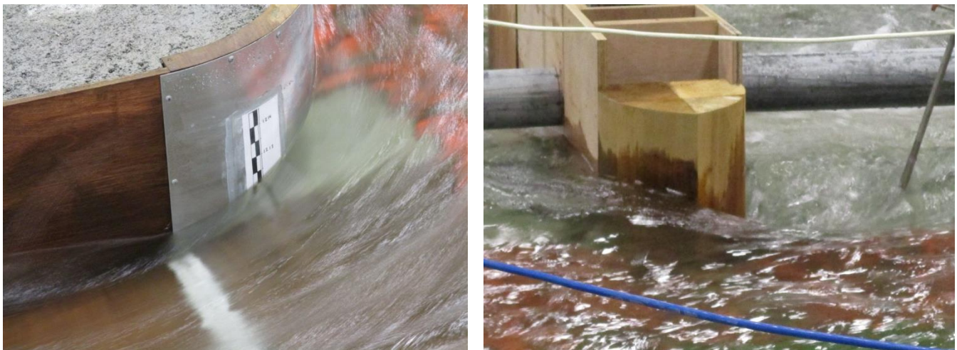
Figure 165. Wakes generated by the retaining wall on the RHS of the service spillway (left), and the RHS of the diversion inlet stemming from pier nose 2 (right).
