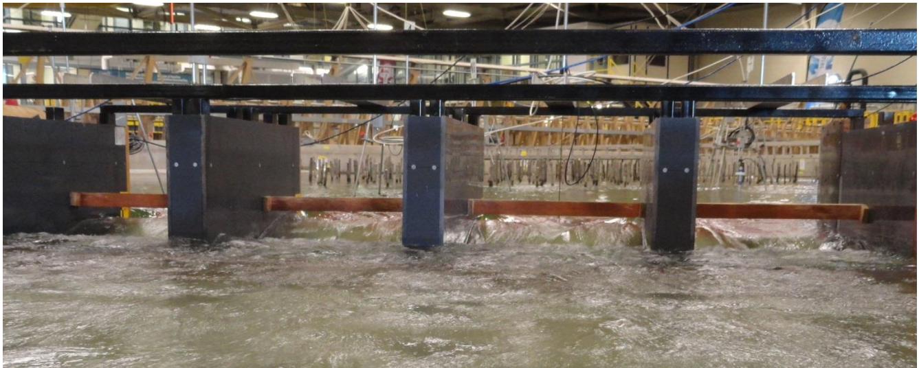
Figure 90. Turbulent flows downstream of diversion inlet gates.
