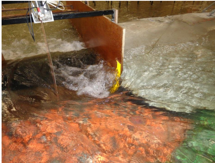
Figure 92. Local flow acceleration and recirculation at the right hand side of the service spillway.
