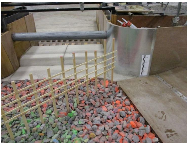
Figure 65. Debris Barrier E implementation in the model.
