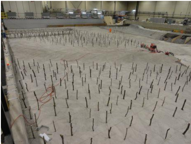
Figure 69. Left – trees cast into the concrete representing the forested floodplain, right – debris rafts in the model including debris with root wad X's at their base.
