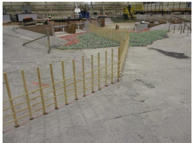
Figure 65. Debris Barrier E implementation in the model.
