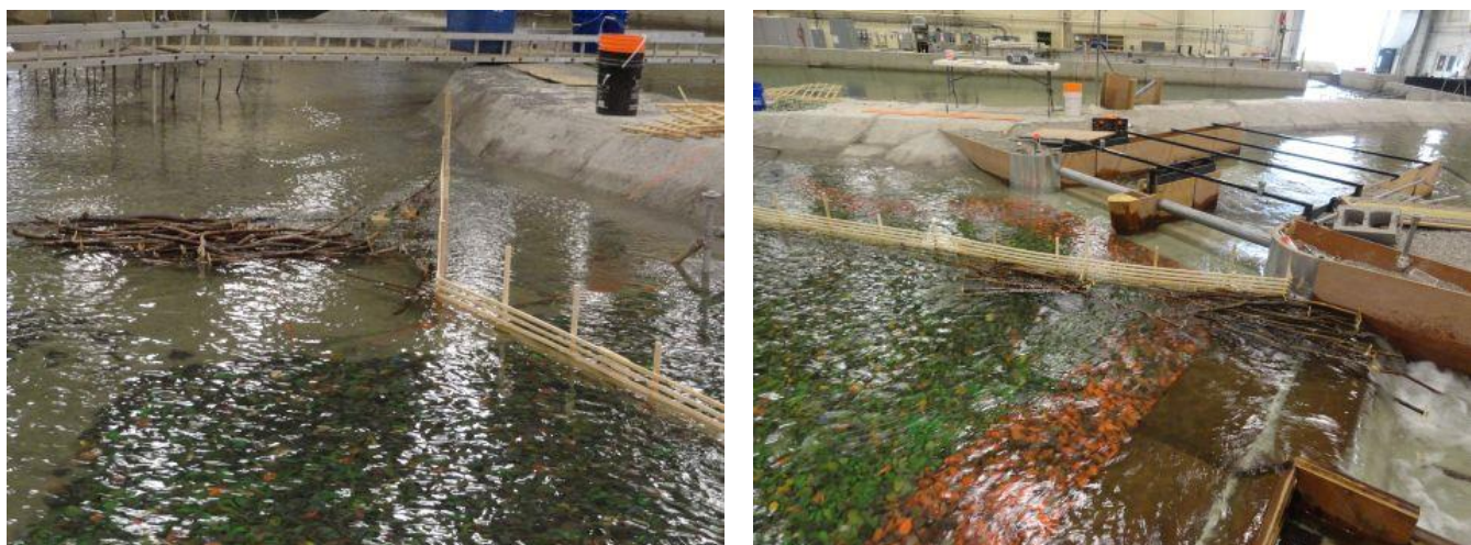
Figure 176. Debris caught on the upstream end of the barrier (leg AB) and protruding out into the river (left), debris caught at the downstream end of the barrier (leg BC) and on the LHS Obermeyer gate (right).
