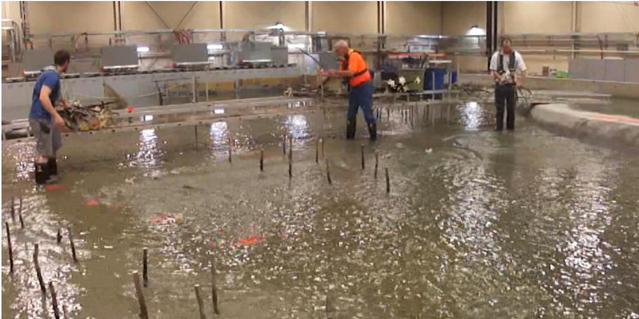
Figure 94. Debris loading locations for 100 trees in 60 seconds.
