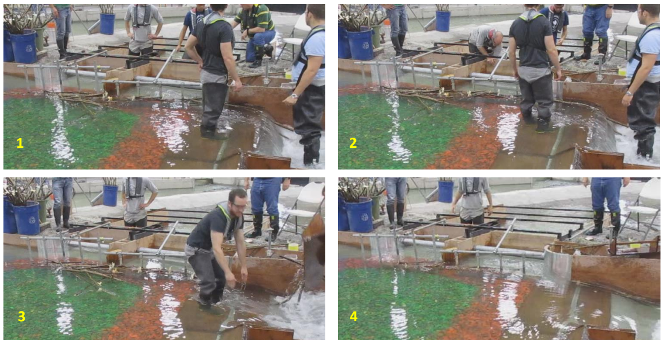
Figure 140. Debris caught on Debris Barrier D , the diversion inlet was closed and LHS Obermeyer gate was lowered to pulse the trees off the barrier.
