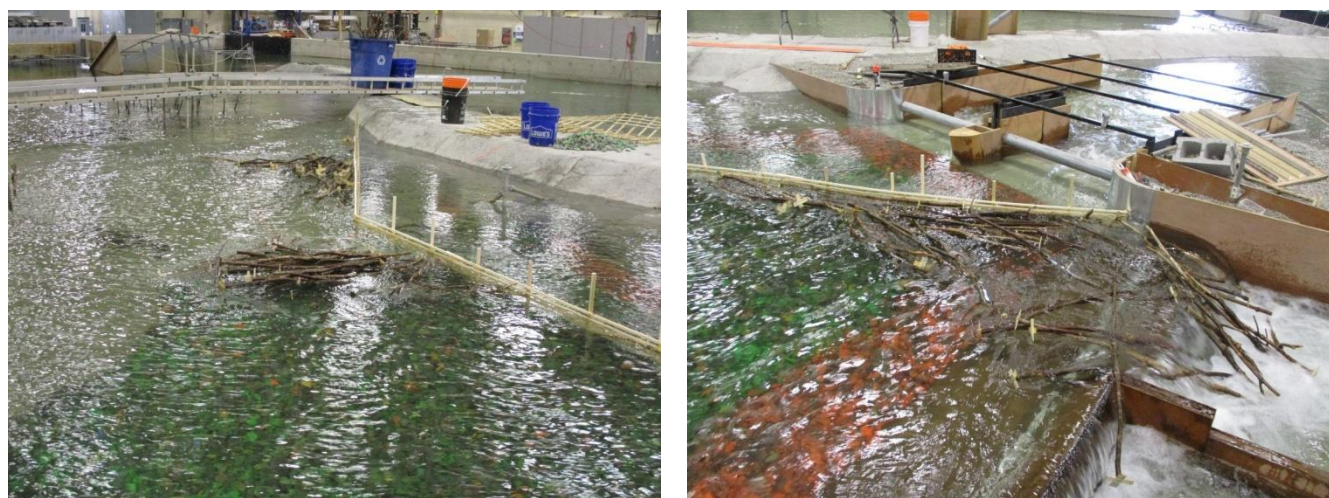
Figure 180. Debris left on barrier at the upstream end (left) and at the end of the barrier bridging across to the central pier in the service spillway (right).
