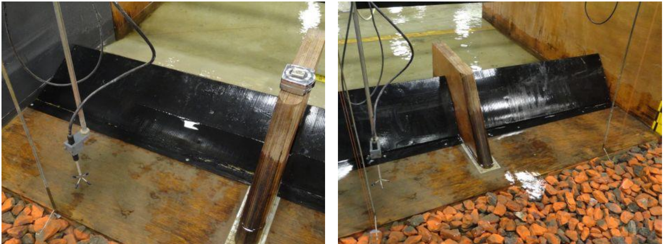
Figure 45. Obermeyer gates were made from sheet metal plate fastened to curved ribs to match the gate profile.
