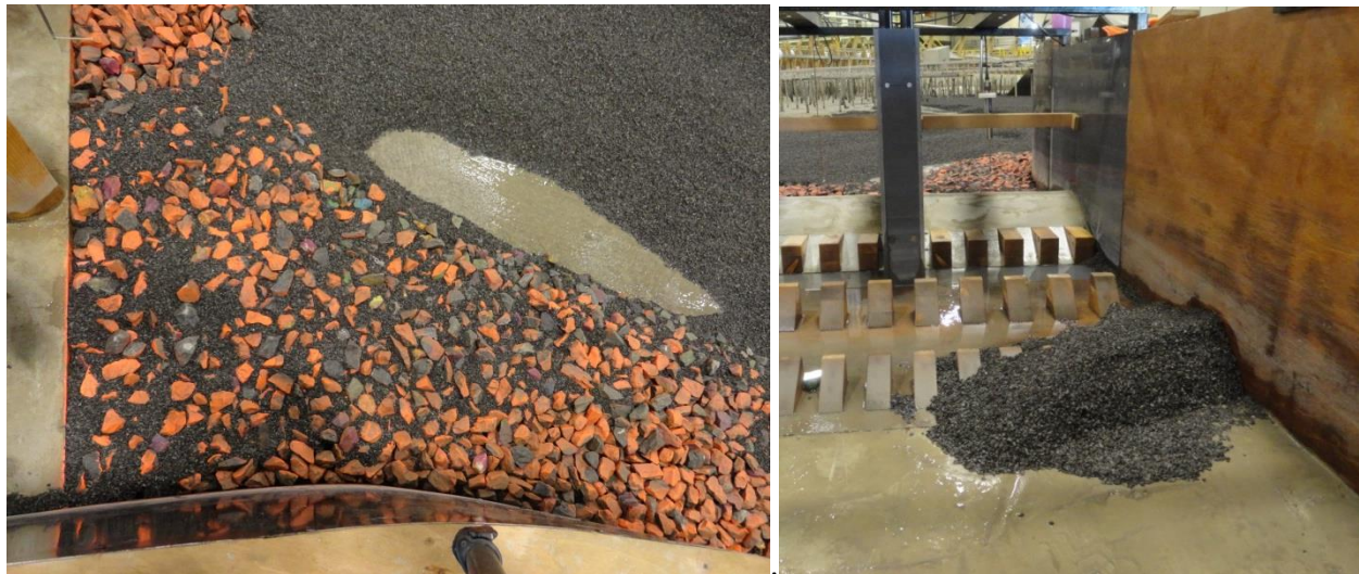
Figure 116. Scour hole on the upstream side of the diversion inlet structure (left) and corresponding sediment deposition on the downstream side (right).
