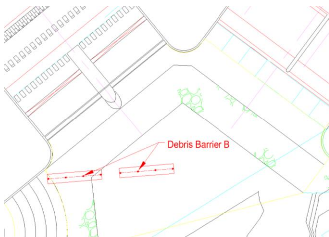
Figure 60. Debris Barrier B layout schematic and implementation in the model.
