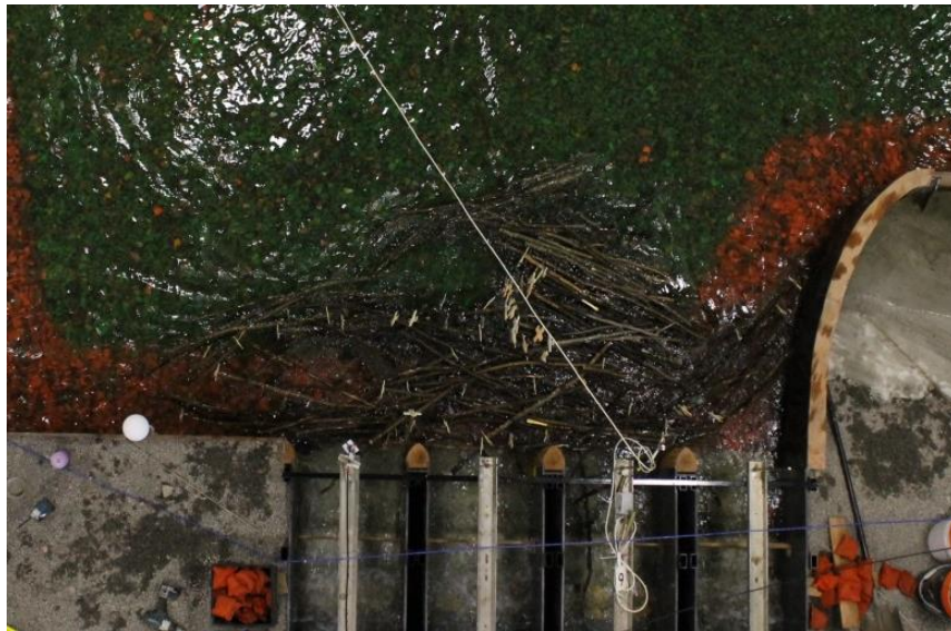
Figure 97. Debris jam of approximately 180 trees.
