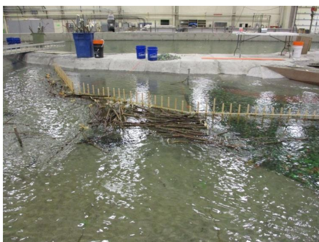
Figure 170. Debris left on barrier at the end of the 760m 3 /s tests for leg AB and BC (left) and at the end of the barrier on leg CD (right).
