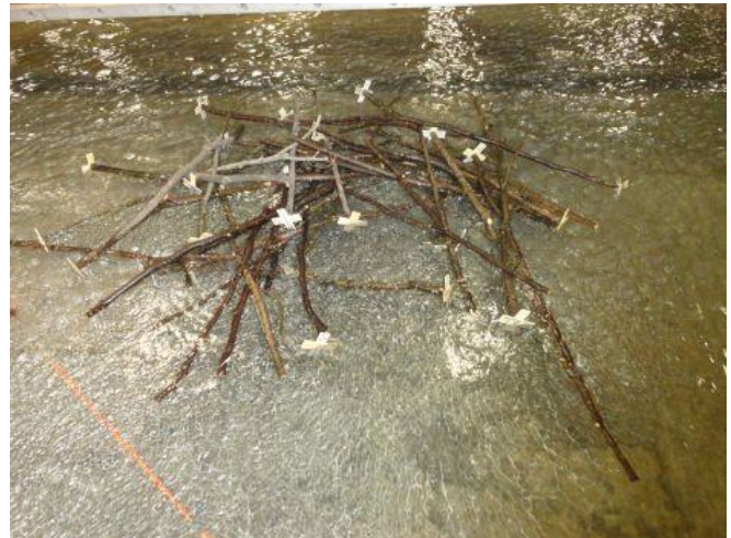
Figure 69. Left – trees cast into the concrete representing the forested floodplain, right – debris rafts in the model including debris with root wad X's at their base.
