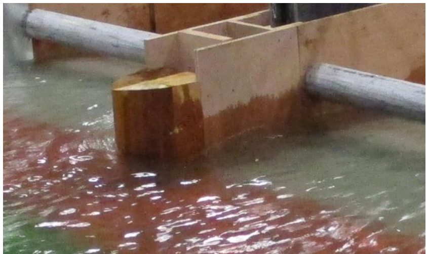
Figure 55. Pier Nose 2 design schematic and implementation in the model.
