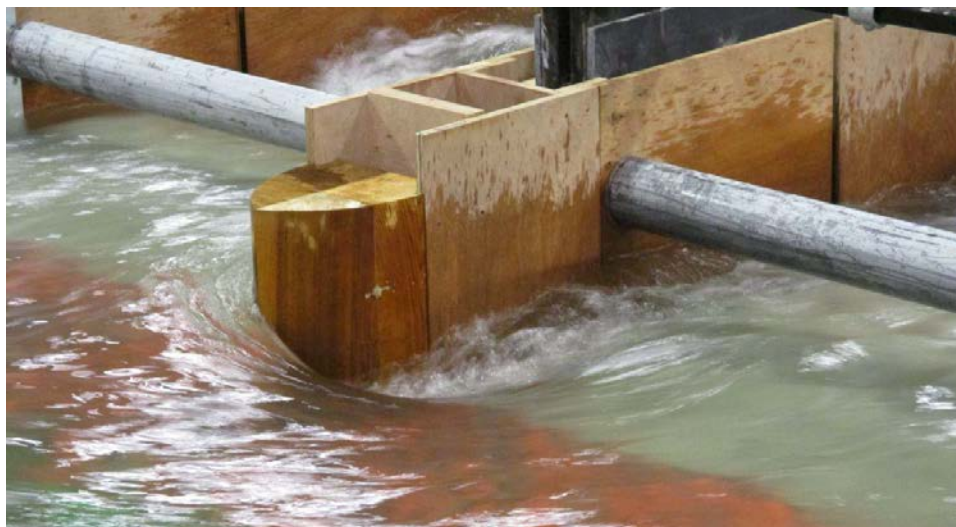
Figure 146. Wake emanating from pier nose 2 during the 1240 m 3 /s event.
