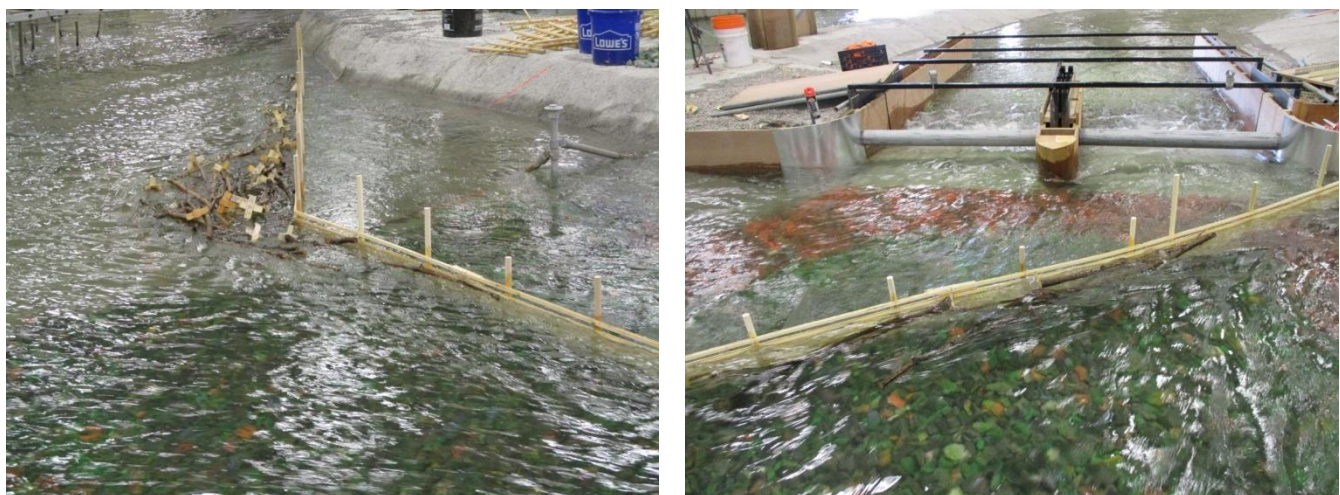
Figure 184. Debris jam at point B (left) and debris caught in the barrier in front of the diversion inlet structure (right) at the end of the TSH tests at 1240m 3 /s.
