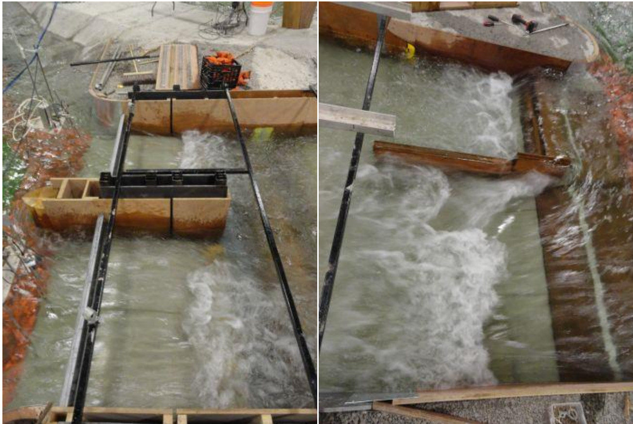
Figure 162. Flow through the diversion inlet structure (left) and service spillway (right) during the 1240m 3 /s case (a) flood condition.
