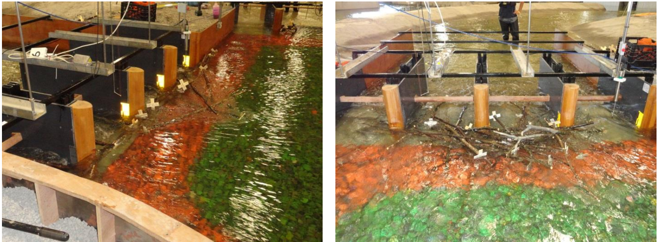
Figure 95. Single trees (left) and a 40-tree raft (right) caught on the diversion inlet piers.
