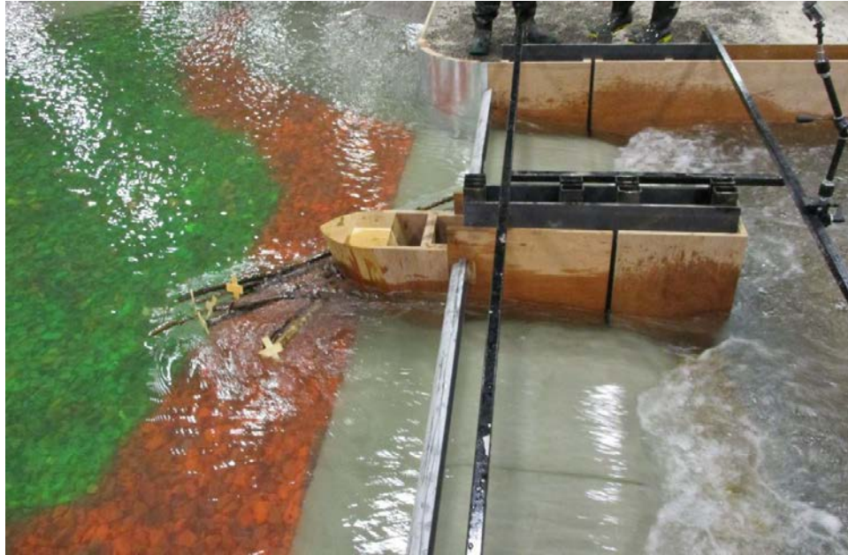
Figure 130. Debris caught on Pier Nose 3.
