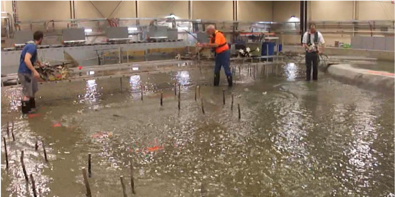
Figure 94. Debris loading locations for 100 trees in 60 seconds.
