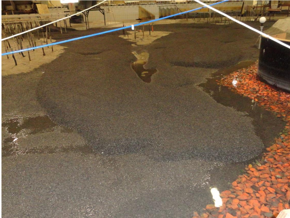
Figure 111. Riverbed in the forebay and upstream areas after the 760 m 3 /s flow condition.
