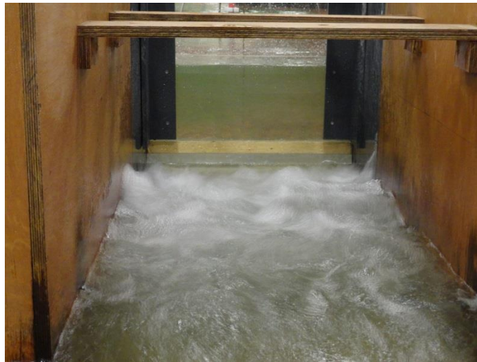
Figure 89. Supercritical flow passing under the sluiceway gate viewed from downstream (with approximately 4.7 m of head on the upstream side of the gate).
