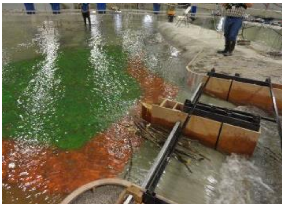
Figure 127. Debris pivoting around Pier Nose 2 while passing through the diversion.
