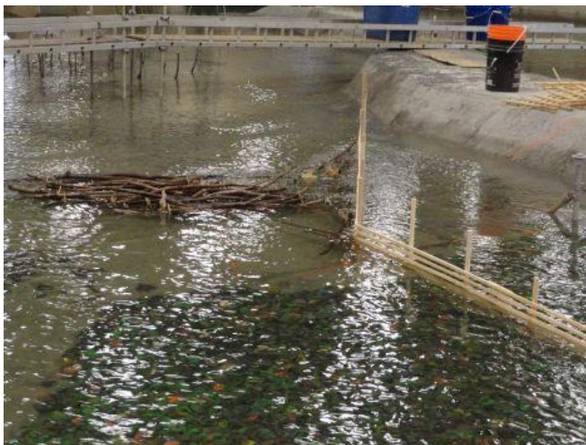
Figure 176. Debris caught on the upstream end of the barrier (leg AB) and protruding out into the river (left), debris caught at the downstream end of the barrier (leg BC) and on the LHS Obermeyer gate (right).
