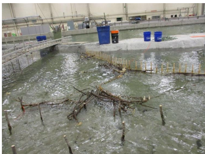
Figure 172. Left - Debris being caught on the barrier and protruding out into the river and this phenomenon continuing to bridge across the river against the standing trees producing a jam. Right – debris trapped in the barrier at the end of the tests.
