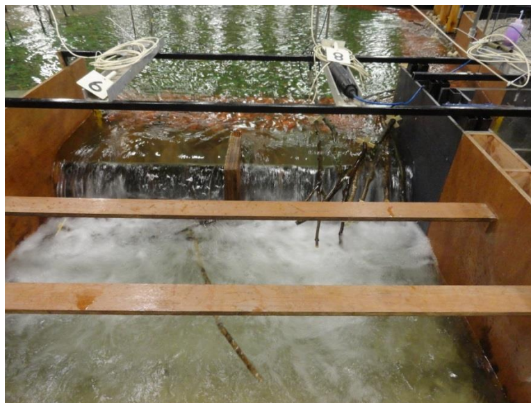
Figure 96. Woody debris caught on the Obermeyer gate and trapped in the downstream roller.
