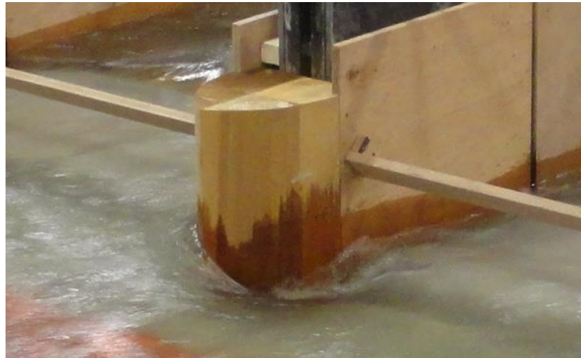
Figure 54. Pier Nose 1 design schematic and implementation in the model.
