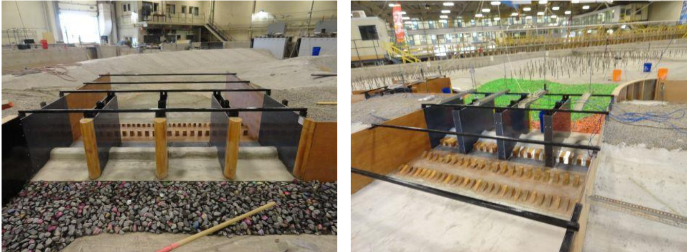
Figure 42. Left: diversion inlet looking downstream. Right: diversion inlet looking upstream (the 440kg riprap and 210kg riprap used in the mobile bed portion of the model was painted to aid in movement detection).
