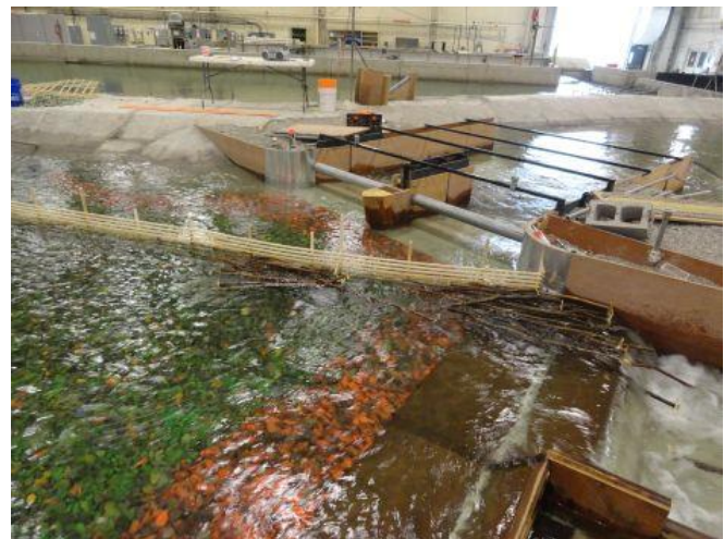
Figure 176. Debris caught on the upstream end of the barrier (leg AB) and protruding out into the river (left), debris caught at the downstream end of the barrier (leg BC) and on the LHS Obermeyer gate (right).
