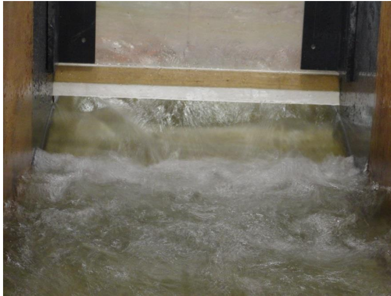
Figure 86. Unobstructed flow passing under the sluiceway gate ( 320 \text{ m}^3/\text{s} ).
