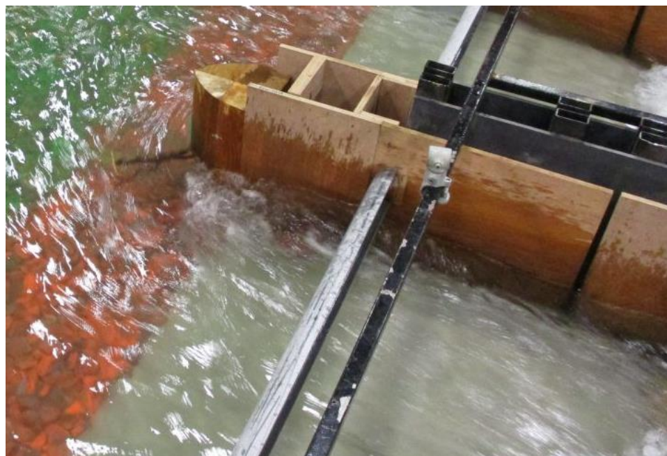
Figure 147. Debris caught on Pier Nose 2.
