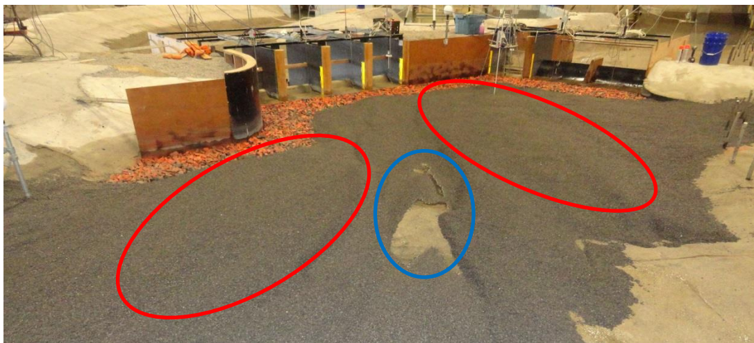
Figure 106. Riverbed morphology in the forebay area following the 320 m 3 /s flow condition; deposition zones in red, erosion zones in blue
