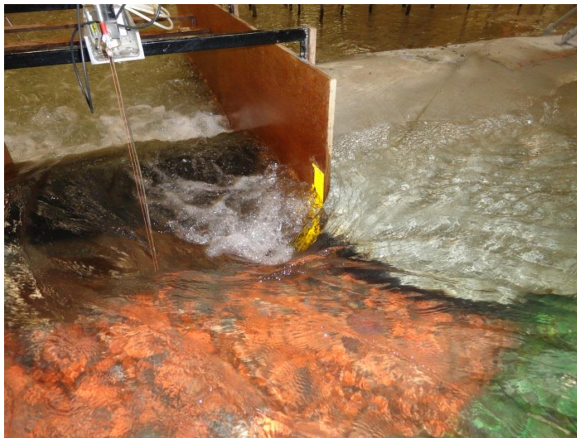
Figure 92. Local flow acceleration and recirculation at the right hand side of the service spillway.
