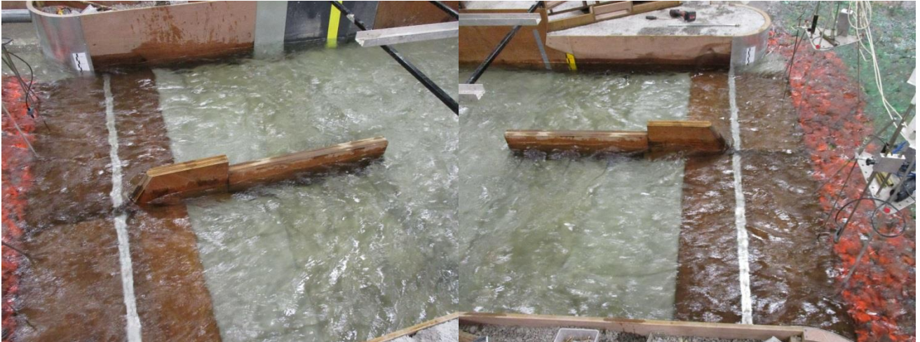
Figure 158. Flow through the service spillway during the 320 m 3 /s case (b) flood condition with the diversion inlet closed.
