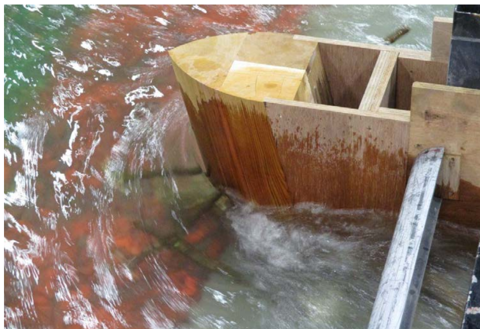
Figure 145. Debris caught on Pier Nose 3.
