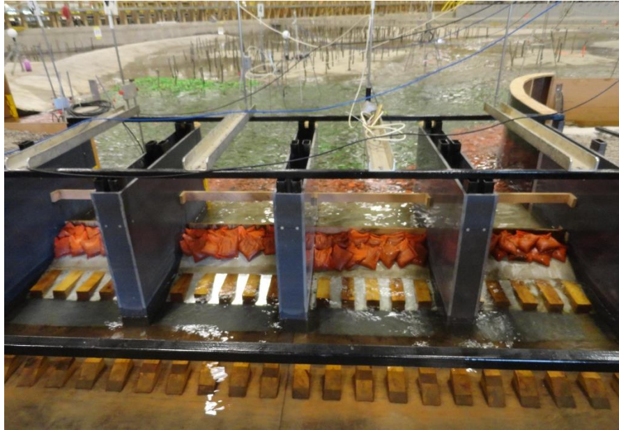
Figure 84. Blockage of the diversion channel inlet for 160 \text{ m}^3/\text{s} flow condition.
