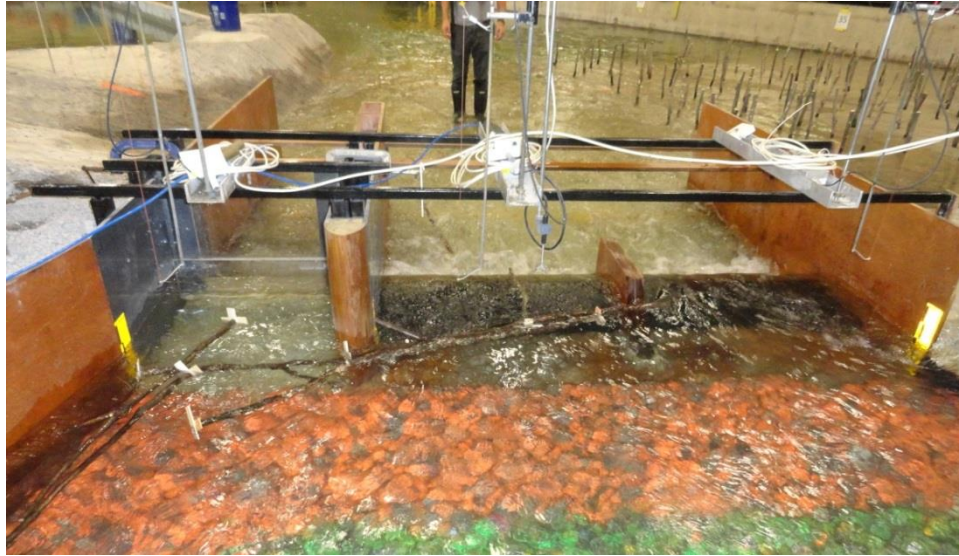
Figure 98. Debris caught in the service spillway/sluiceway with lower (1211.8m) Obermeyer gate setting.
