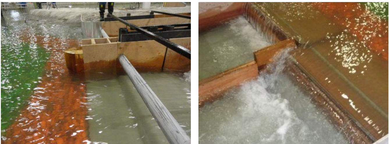
Figure 126. Flow conditions at the structure during the 760 m 3 /s event with the Obermeyer gates set to 1213.4m (LHS) and 1215m (RHS) and Pier Nose 2 installed. Left - facing southwest at the diversion, right - facing southeast at the service spillway.
