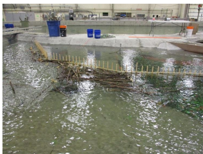
Figure 170. Debris left on barrier at the end of the 760m 3 /s tests for leg AB and BC (left) and at the end of the barrier on leg CD (right).
