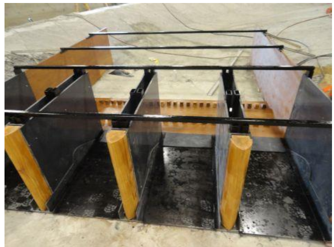
Figure 39. Left: installing the pier noses. Right: installing the support struts, rear retaining walls and rear stilling basin chute blocks.
