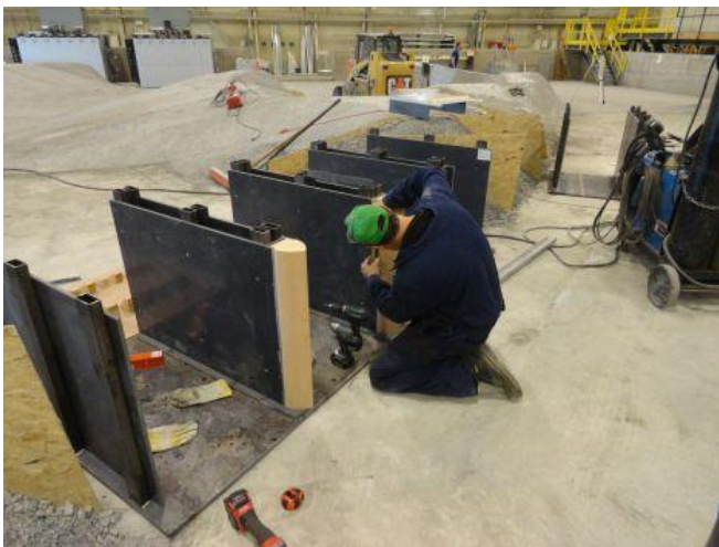
Figure 39. Left: installing the pier noses. Right: installing the support struts, rear retaining walls and rear stilling basin chute blocks.
