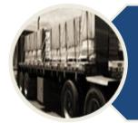
For tiedowns that go from one anchor point to another on the vehicle, add the WLLs of each tiedown to get the aggregate WLL of the load.
