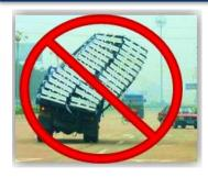
Each tiedown must be secured so that it does not come loose, unfastened, opened or released while the vehicle is moving. This means that the driver of a vehicle must be able to securely tighten a tiedown before transporting their cargo on a highway.
