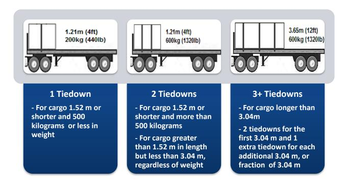
When a piece of cargo is not blocked or positioned to prevent forward movement:
