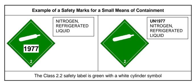
All large means of containment, including a vehicle acting as a large means of containment, must be clearly marked with four Class 2.2 placards, one on each of the four sides of the large means of containment or vehicle [Section 4.15]. The UN number must be shown inside each placard or on an adjacent orange panel [Section 4.8].
