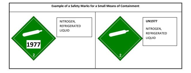
Class 2.2 Non-Flammable and Non-Toxic Gases safety label is green with a white gas cylinder symbol
