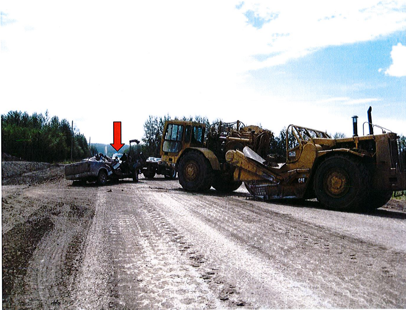
Photograph 3 Shows the Foreman's _____ truck after it had collided with the front left side of the scraper. The area of impact was directly to the passenger side of the pickup truck.
